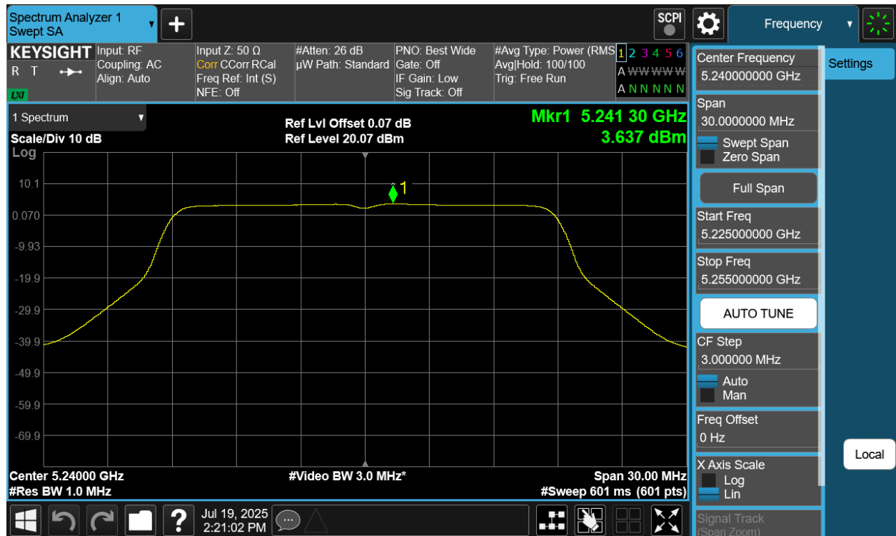
Plot 7-69 PSD CDD Primary Antenna WF5B (20MHz BW 802.11 - Ch.48)
