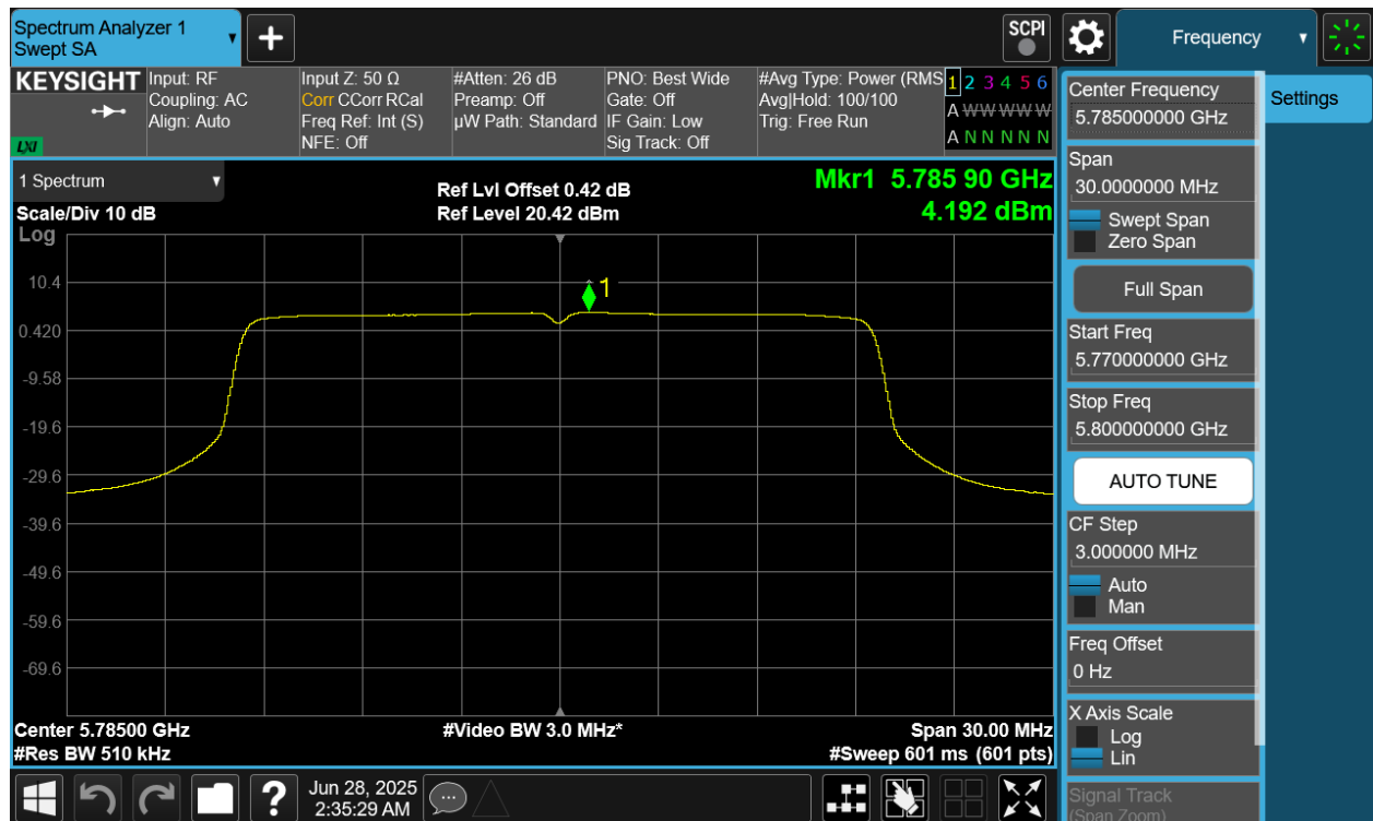
Plot 7-88 PSD CDD Diversity Antenna 2a (20MHz BW 802.11be(SU) - Ch.157)
