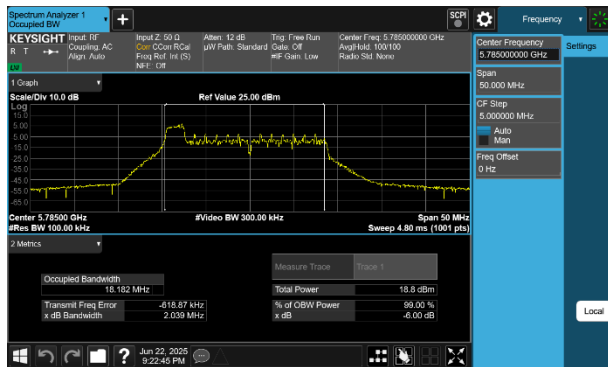
Plot 7-34 6dB BW & 99% OBW Antenna WF5B (20MHz BW 802.11be(RU) RU26 Index0 - Ch.157)
