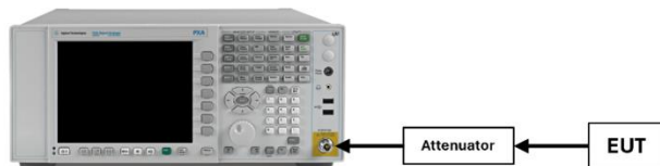
Figure 7-4. Test Instrument & Measurement Setup
