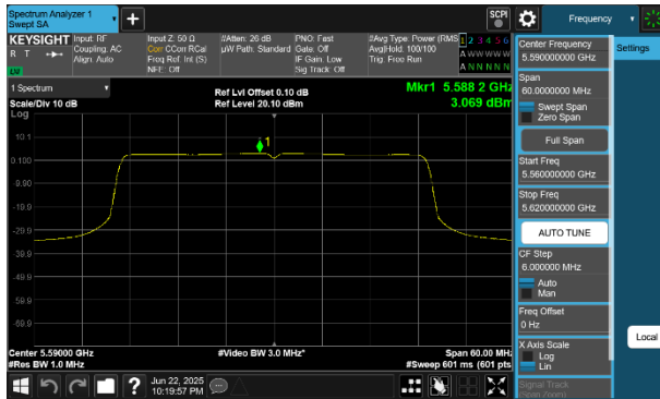
Plot 7-66 PSD Antenna WF5B (40MHz BW 802.11be(RU) RU484 Index65 - Ch.118 (FCC ONLY))
