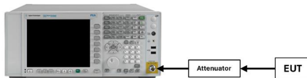
Figure 7-1. Test Instrument & Measurement Setup
