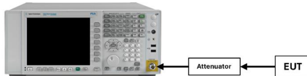
Figure 7-2. Test Instrument & Measurement Setup
