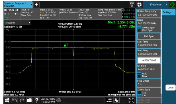
Plot 7-68 PSD Antenna WF5B (160MHz BW 802.11be(RU) RU996X2 Index68 - Ch.114)
