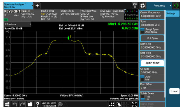
Plot 7-62 PSD Antenna WF5B (20MHz BW 802.11be(RU) RU52+26 Index71 - Ch.60)
