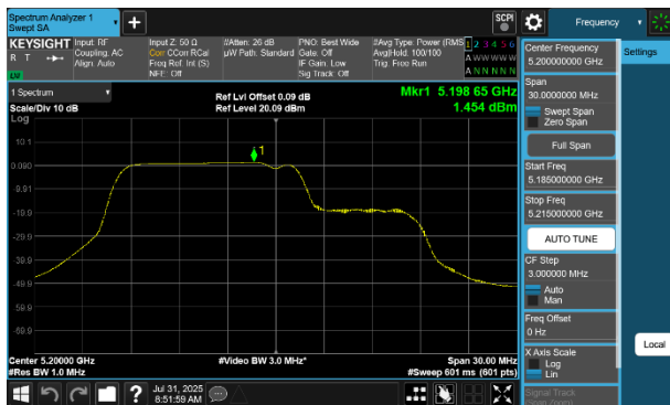
Plot 7-254 PSD SDM Diversity Antenna 2a (20MHz BW 802.11be(RU) RU106+26 Index82 - Ch.40)
