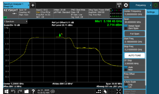
Plot 7-257 PSD SDM Diversity Antenna 4a (20MHz BW 802.11be(RU) RU106+26 Index82 - Ch.40)
