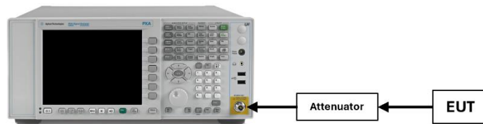
Figure 7-4. Test Instrument & Measurement Setup
