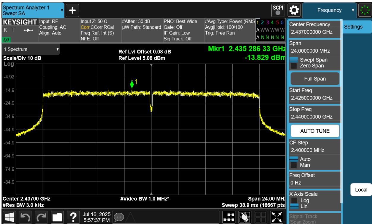
Plot 7-22 PSD CDD Antenna 2a (20MHz BW 802.11be(RU) RU242 Index61 - Ch.6)
