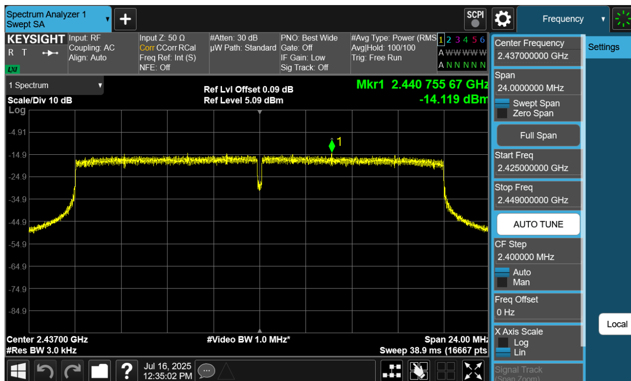
Plot 7-14 PSD Antenna 2a (20MHz BW 802.11be(RU) RU242 Index61 - Ch.6)
