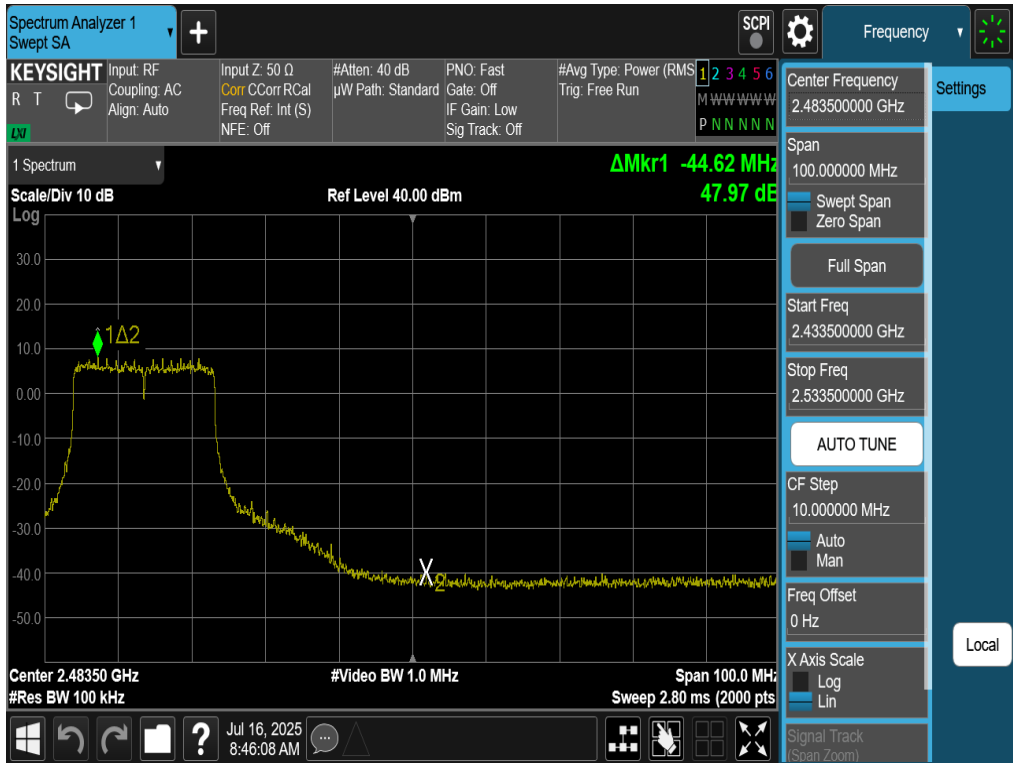
Plot 7-37. Band Edge Antenna 4a (802.11be OFDMA – RU242 – Ch. 8)
