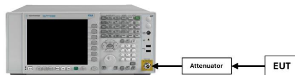
Figure 7-5. Test Instrument & Measurement Setup
