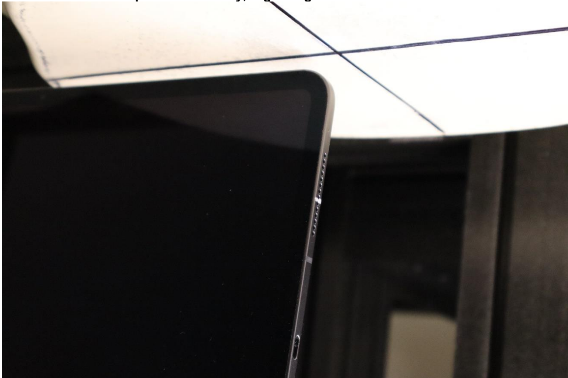
SAR Test Setup Photo 10: Body, Right Edge at 5mm – Antenna 1/2a/2b/WF5B
