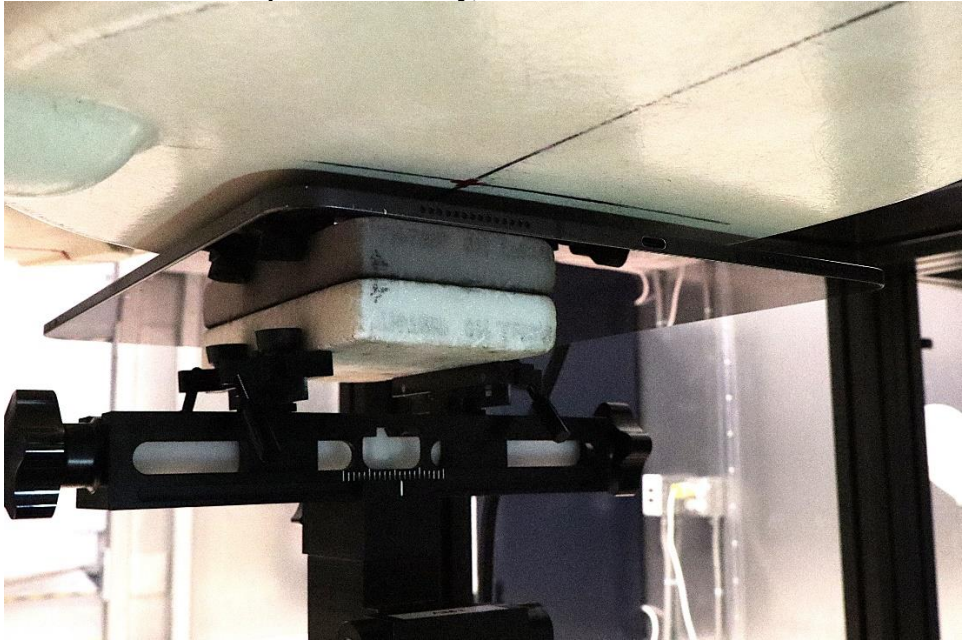
SAR Test Setup Photo 3: Body, Back Side at 5mm– Antenna 2b
