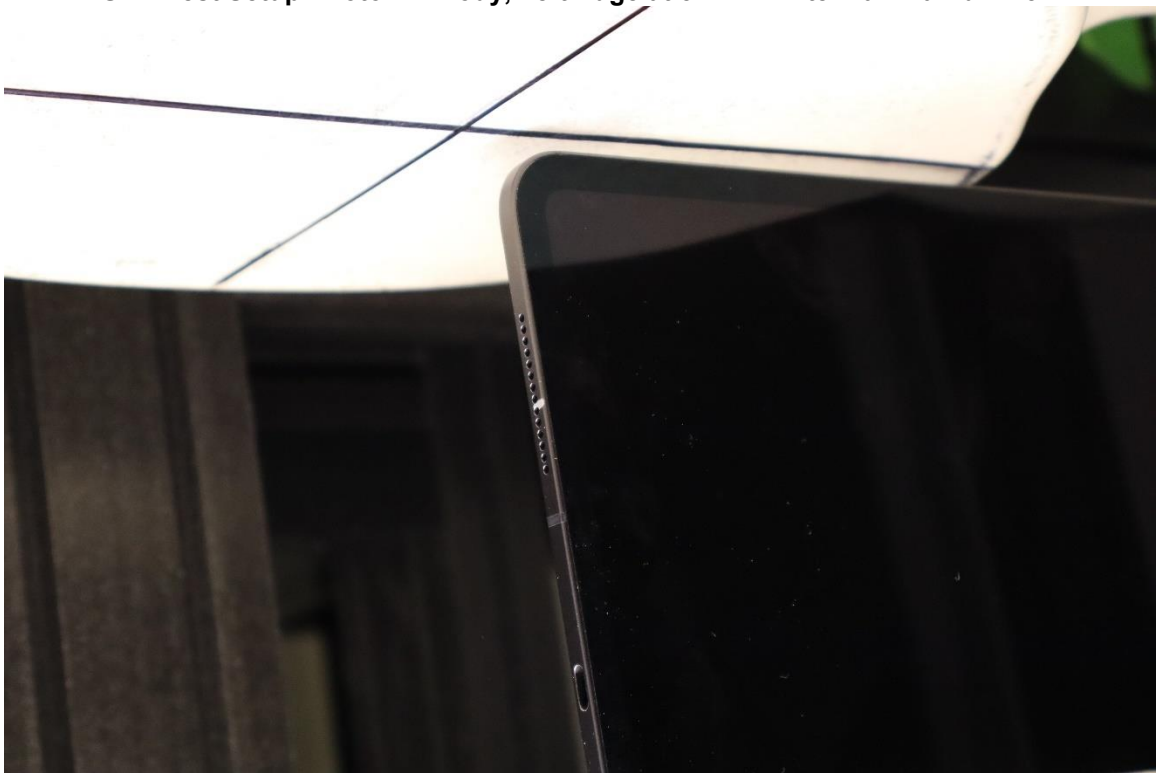
SAR Test Setup Photo 12: Body, Left Edge at 5mm – Antenna 1/2a/2b/WF5B
