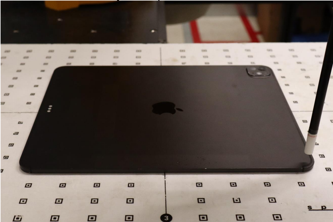
Near Field Power Density Test Setup 22: Back Side at 9.00mm – Antenna 4a
