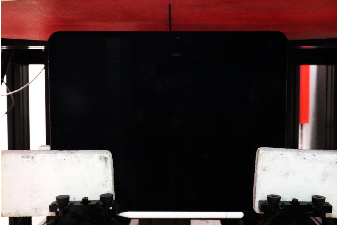
Wireless Power Transfer (WPT) Test Setup Photo 17: Left Edge at 5mm
