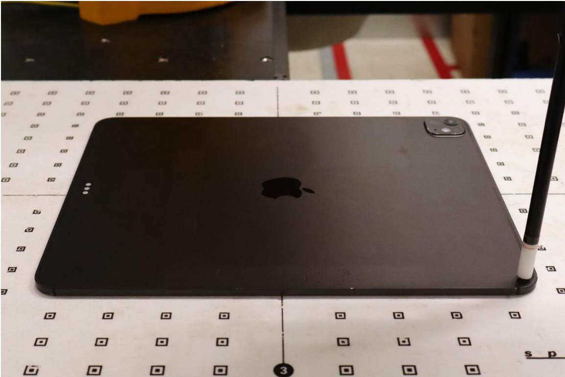
Near Field Power Density Test Setup 21: Back Side at 2mm – Antenna 4a
