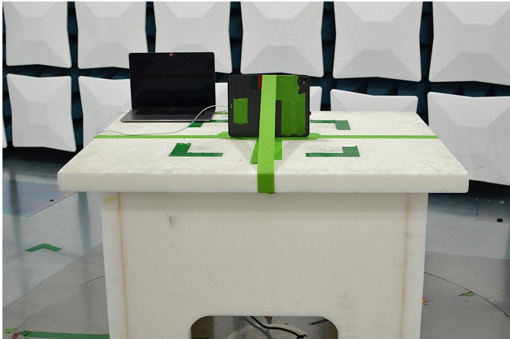
Figure 15: 30MHz-1GHz Test Setup (Front View)
