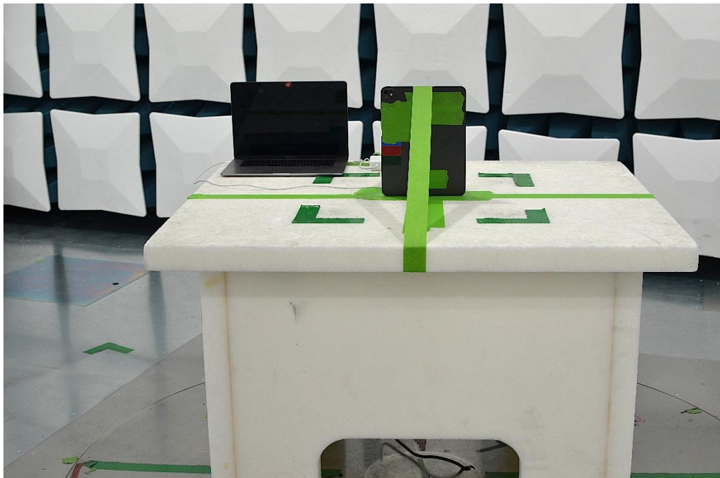
Figure 17: 30MHz-1GHz Test Setup (Front View)
