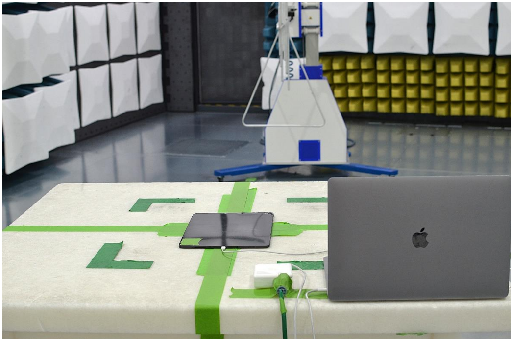
Figure 14: 30MHz-1GHz Test Setup (Rear View)
