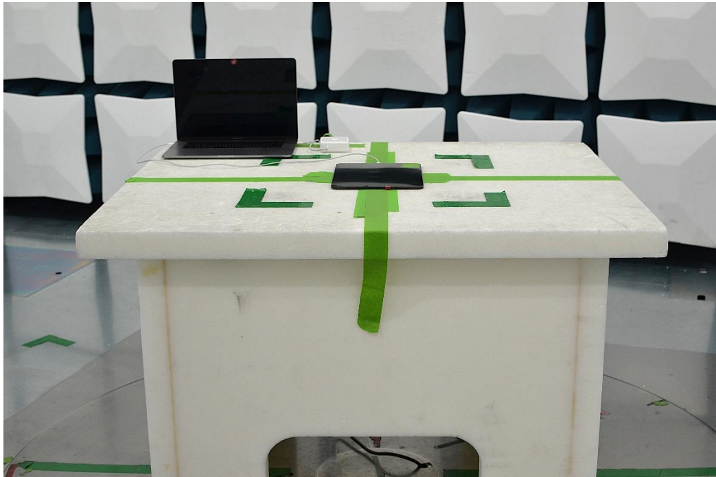
Figure 13: 30MHz-1GHz Test Setup (Front View)
