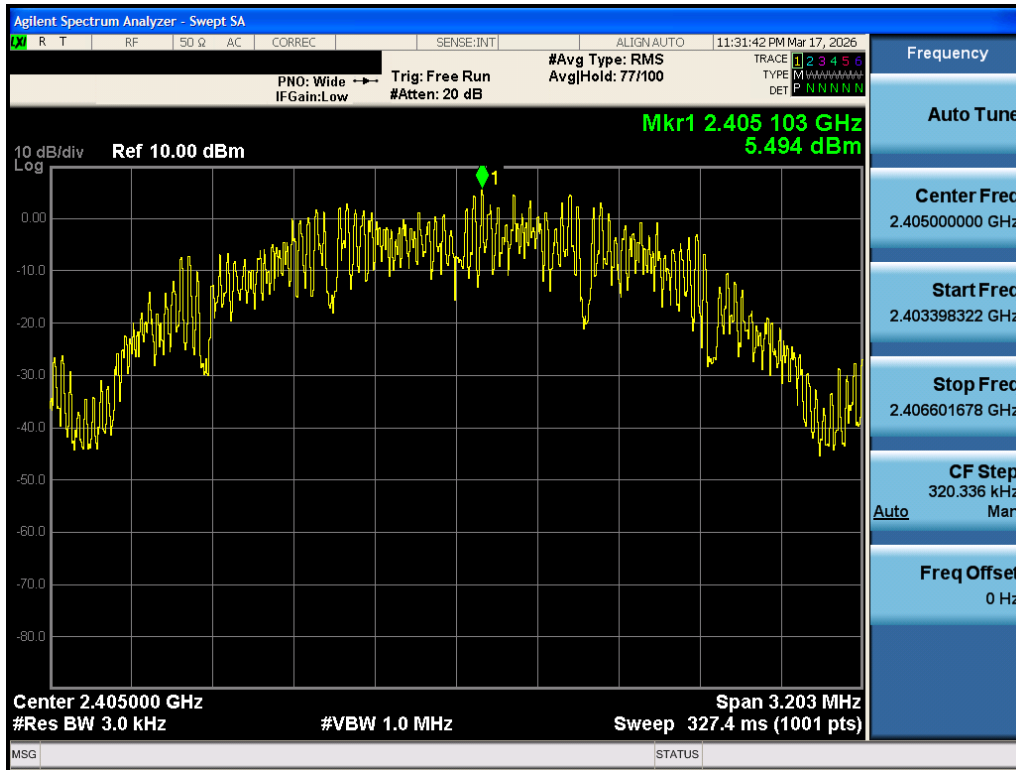
Plot 7-13. Power Spectral Density Antenna 1 Dedicated (802.15.4, ePA – Ch. 11)
