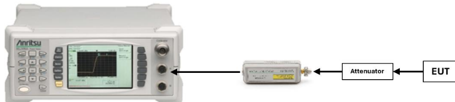
Figure 7-3. Test Instrument & Measurement Setup for Peak and Average Power Measurement
