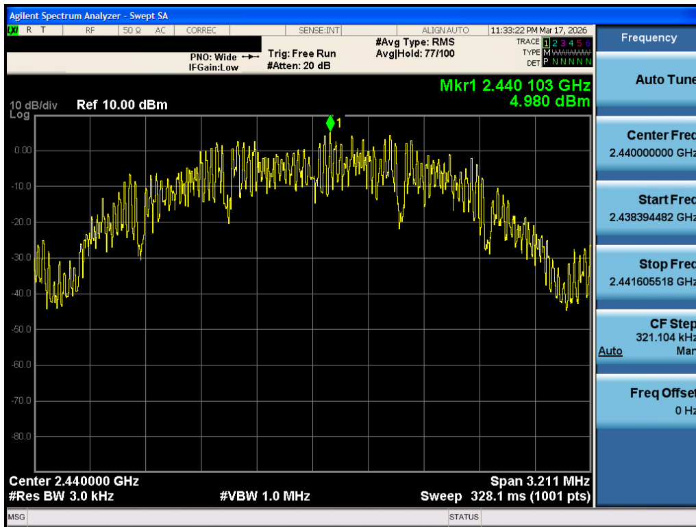
Plot 7-14. Power Spectral Density Antenna 1 Dedicated (802.15.4, ePA – Ch. 18)
