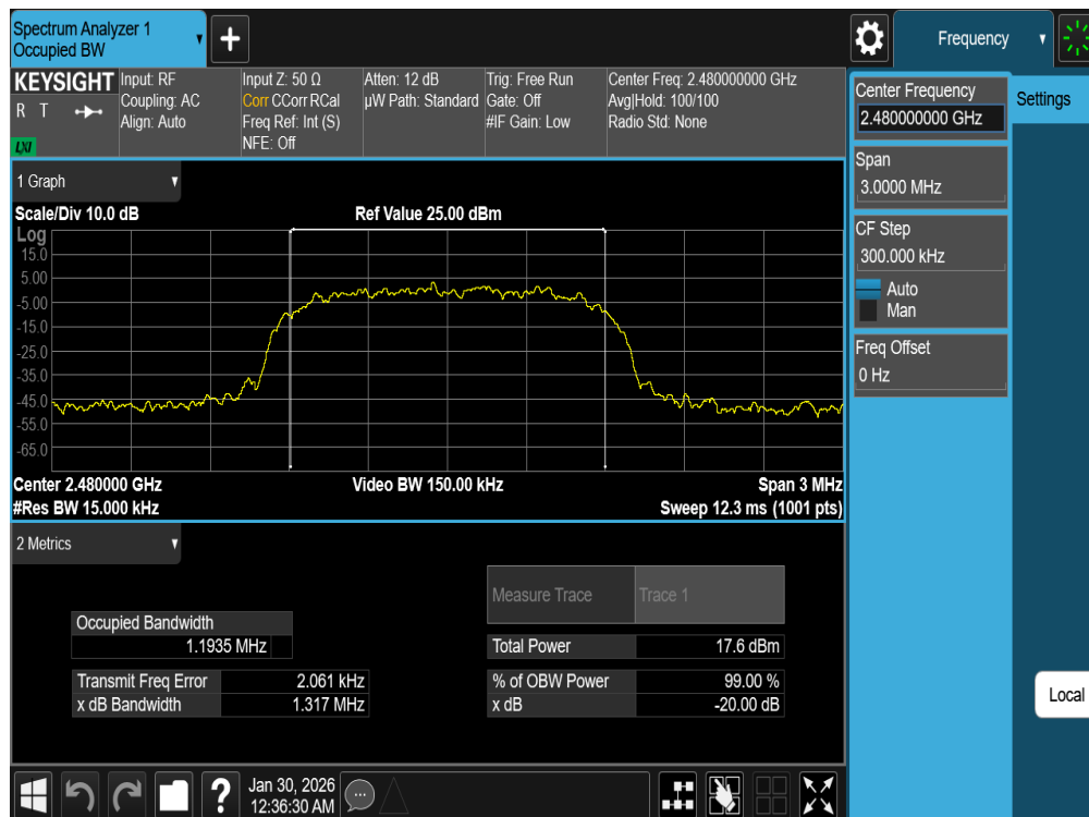
Plot 7-6. 20dB BW and 99% OBW Plot Antenna 0 (Bluetooth, 8DPSK, iPA – Ch. 78)
