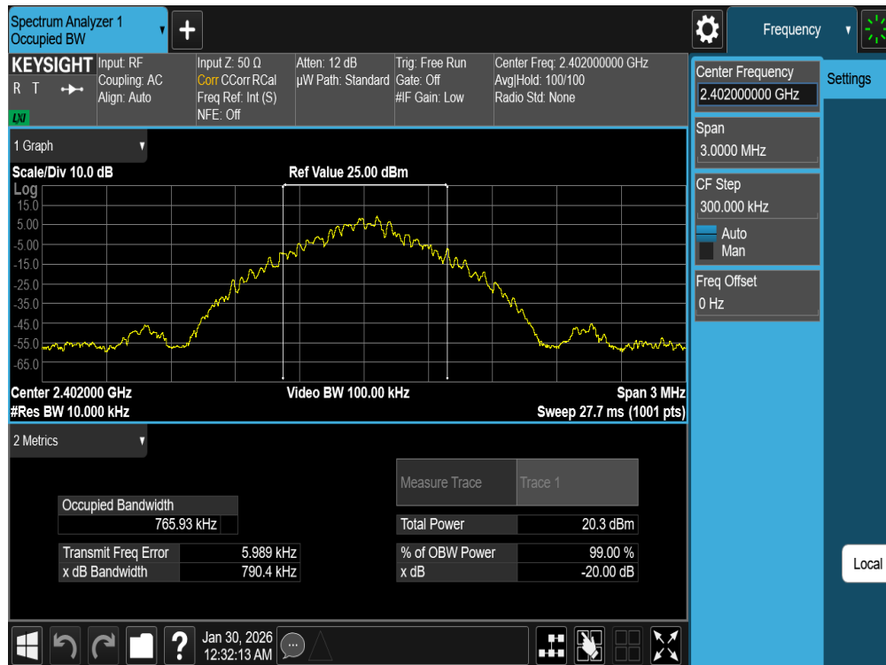
Plot 7-1. 20dB BW and 99% OBW Plot Antenna 0 (Bluetooth, GFSK, iPA – Ch. 0)
