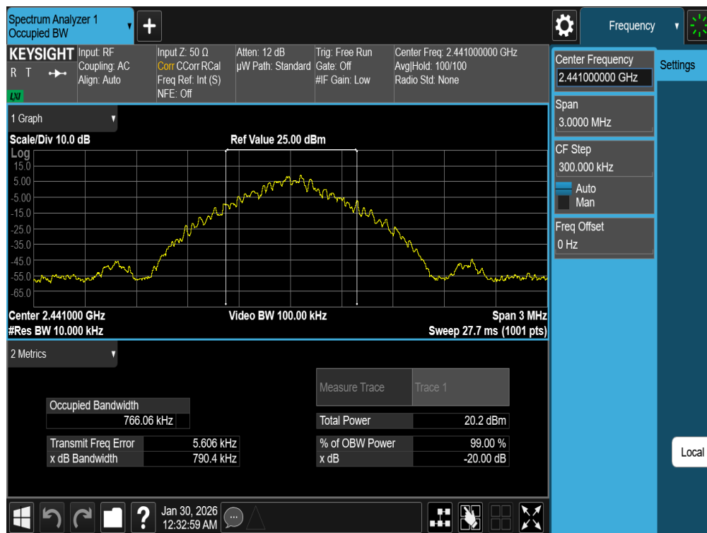
Plot 7-2. 20dB BW and 99% OBW Plot Antenna 0 (Bluetooth, GFSK, iPA – Ch. 39)
