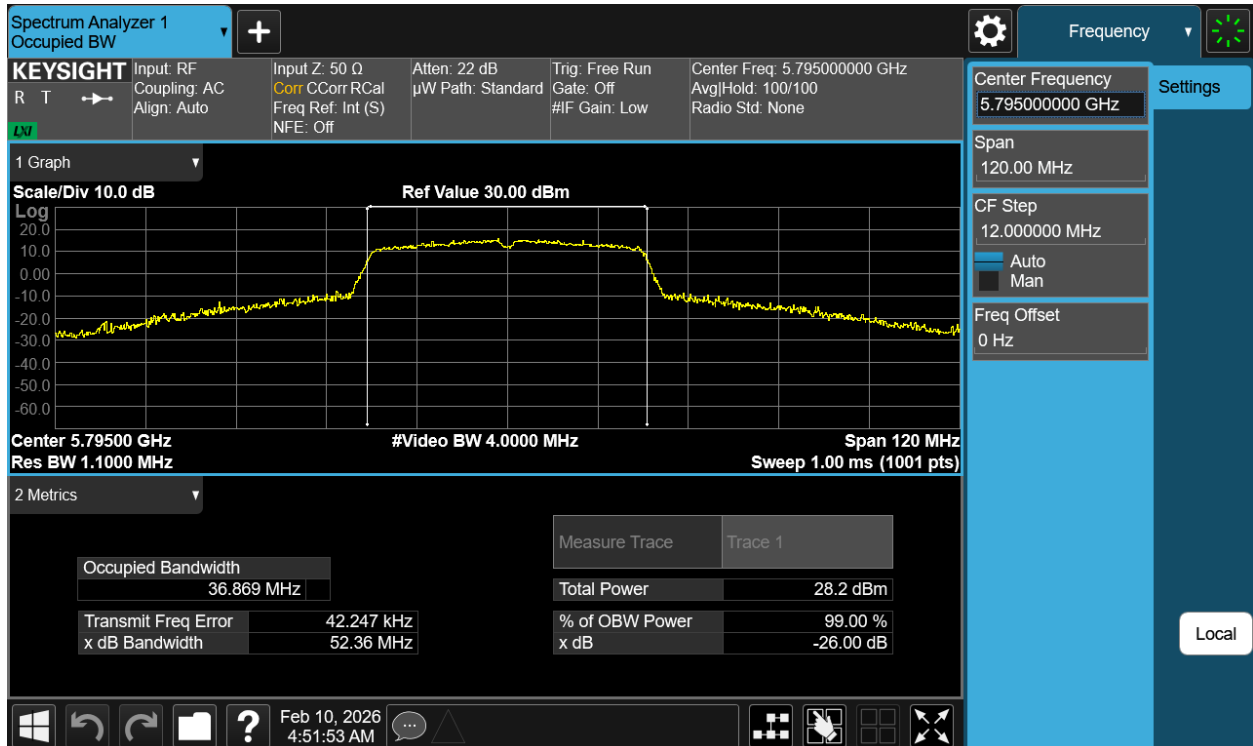
Plot 7-5 99% OBW Antenna 0 (40MHz BW 802.11n - Ch.159)
