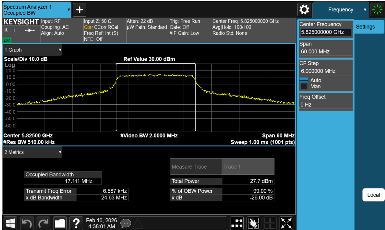
Plot 7-4 99% OBW Antenna 0 (20MHz BW 802.11a - Ch.165)
