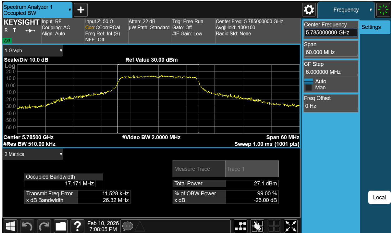
Plot 7-10 99% OBW Antenna 1 (20MHz BW 802.11a - Ch.157)
