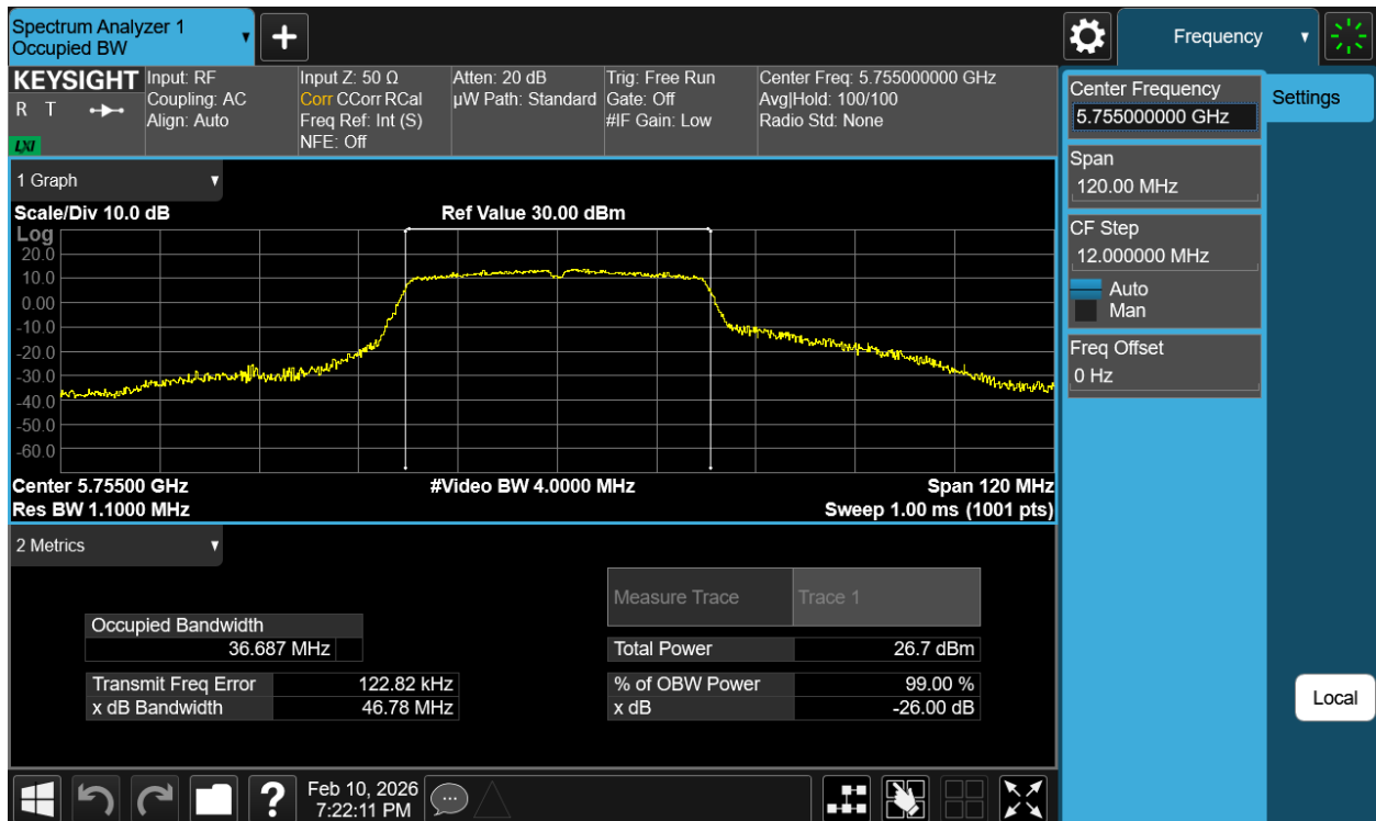
Plot 7-11 99% OBW Antenna 1 (40MHz BW 802.11n - Ch.151)
