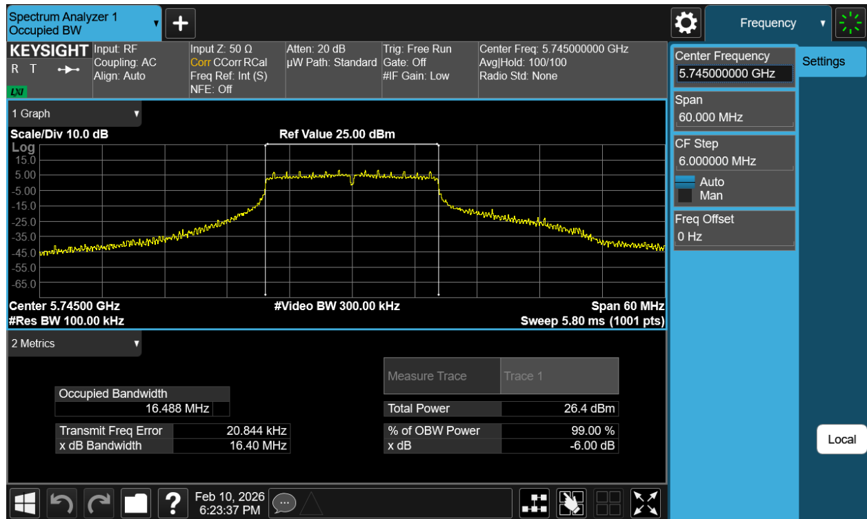
Plot 7-16 6dB OBW Antenna 1 (20MHz BW 802.11a - Ch.149)
