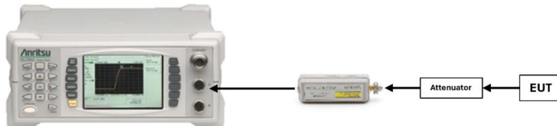
Figure 7-3. Test Instrument & Measurement Setup
