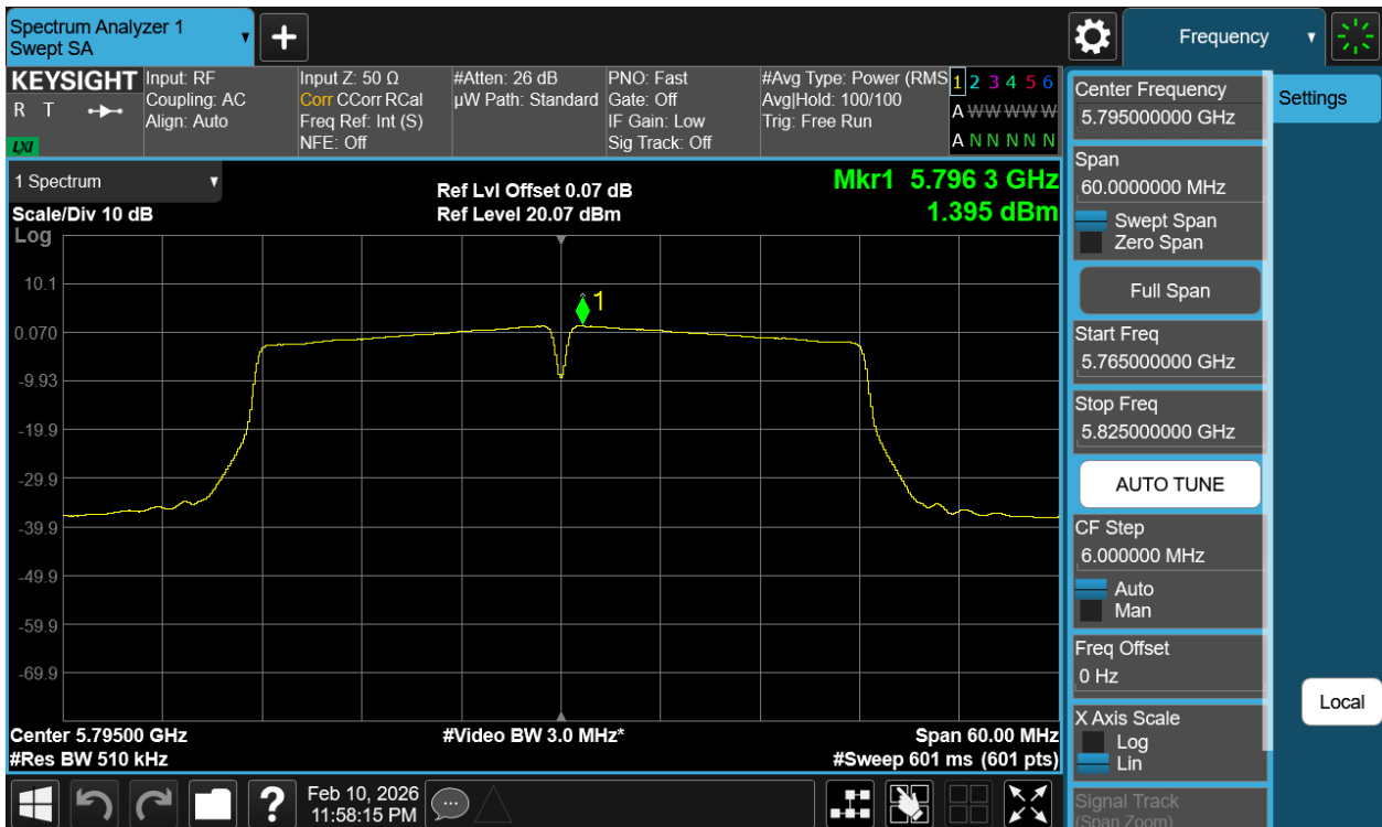
Plot 7-32 PSD Antenna 1 (40MHz BW 802.11n - Ch.159)
