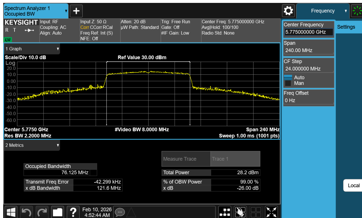
Plot 7-6 99% OBW Antenna 0 (80MHz BW 802.11ac - Ch.155)
