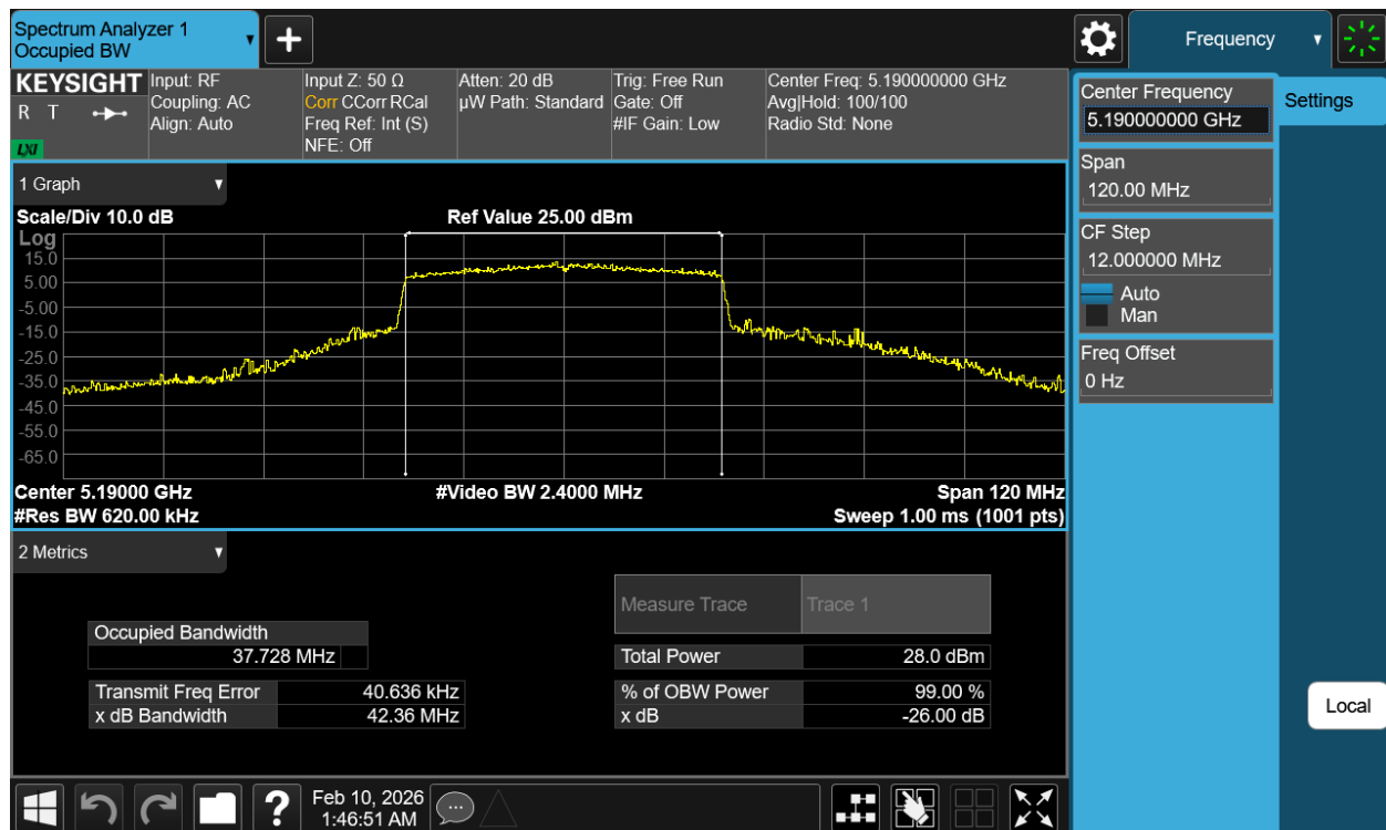
Plot 7-2 26dB BW & 99% OBW Antenna 0 (40MHz BW 802.11ax(SU) - Ch.38)
