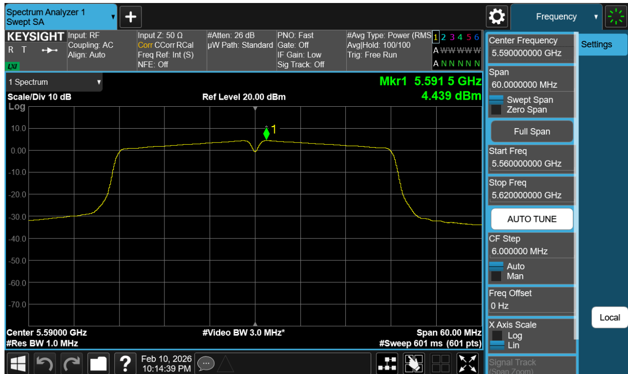
Plot 7-29 PSD Antenna 1 (40MHz BW 802.11n - Ch.118)
