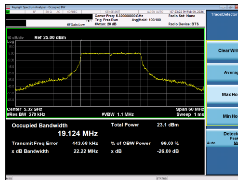
Plot 7-4 26dB BW & 99% OBW Antenna 0 (20MHz BW 802.11ax(RU) RU242 Index61 - Ch.64)
