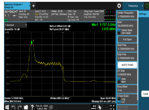
Plot 7-76 PSD CDD Antenna 1 (40MHz BW 802.11ax(RU) RU26 Index0 - Ch.151)
