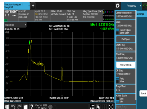
Plot 7-78 PSD CDD Antenna 1 (80MHz BW 802.11ax(RU) RU26 Index0 - Ch.155)
