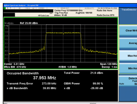
Plot 7-5 26dB BW & 99% OBW Antenna 0 (40MHz BW 802.11ax(RU) RU484 Index65 - Ch.102)
