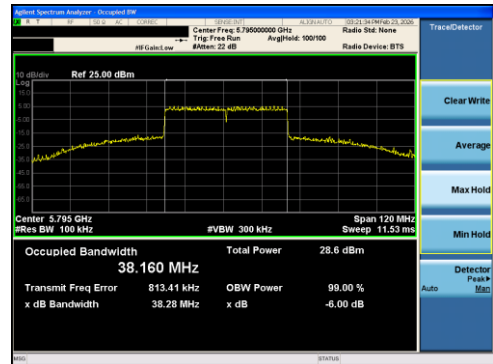
Plot 7-23 6dB OBW Antenna 1 (40MHz BW 802.11ax(RU) RU484 Index65 - Ch.159)
