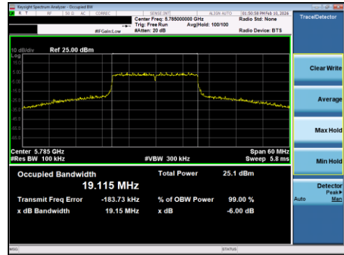
Plot 7-22 6dB OBW Antenna 1 (20MHz BW 802.11ax(RU) RU242 Index61 - Ch.157)
