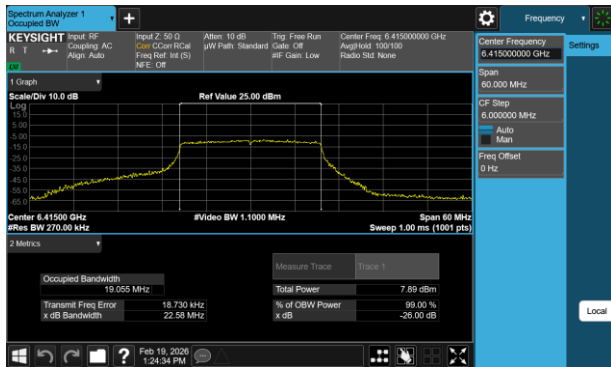
Plot 7-13 26dB BW & 99% OBW Antenna 1 (20MHz BW 802.11ax(SU) - Ch.93)
