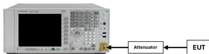
Figure 7-4. Test Instrument & Measurement Setup
