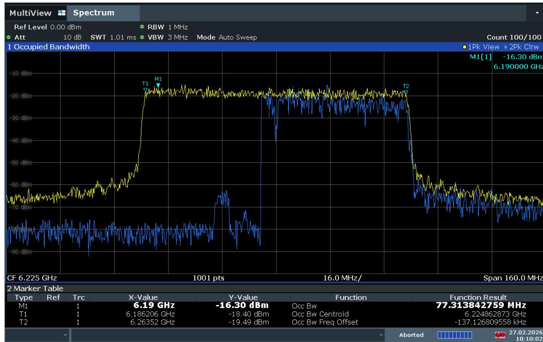
Plot 7-244. 80MHz Bandwidth, AWGN Signal Injected – 6190Mhz
