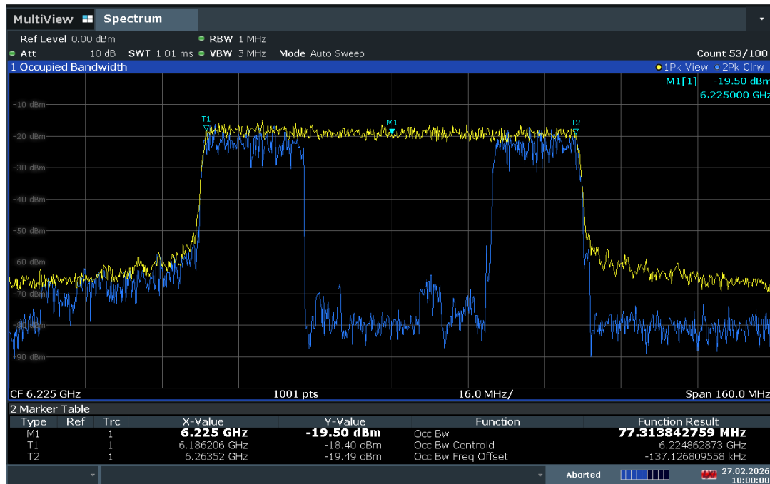
Plot 7-245. 80MHz Bandwidth, AWGN Signal Injected – 6225MHz
