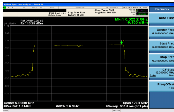
Plot 7-150 PSD Antenna 1 (80MHz BW 802.11ax(RU) RU996 Index67 - Ch.7)
