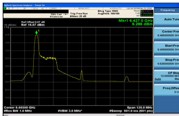
Plot 7-93 PSD Antenna 0 (80MHz BW 802.11ax(RU) RU26 Index0 - Ch.103)
