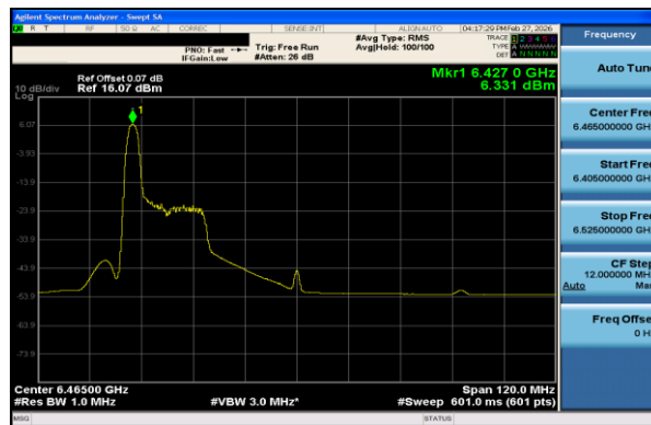
Plot 7-135 PSD Antenna 1 (80MHz BW 802.11ax(RU) RU26 Index0 - Ch.103)
