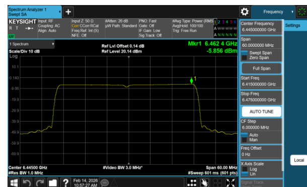
Plot 7-113 PSD Antenna 0 (40MHz BW 802.11ax(RU) RU484 Index65 - Ch.99)
