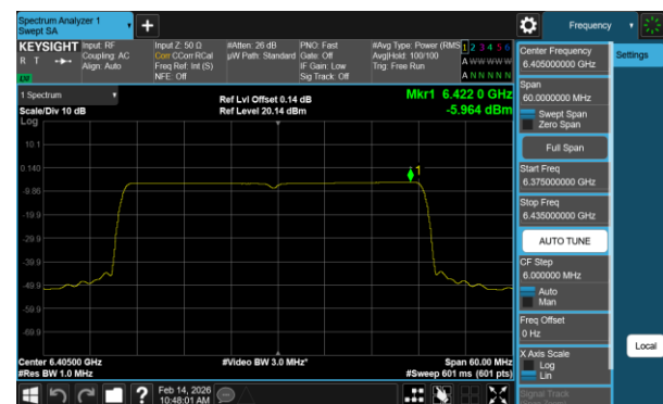
Plot 7-107 PSD Antenna 0 (40MHz BW 802.11ax(RU) RU484 Index65 - Ch.91)
