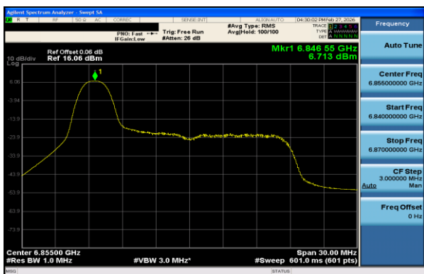
Plot 7-139 PSD Antenna 1 (20MHz BW 802.11ax(RU) RU26 Index0 - Ch.181)
