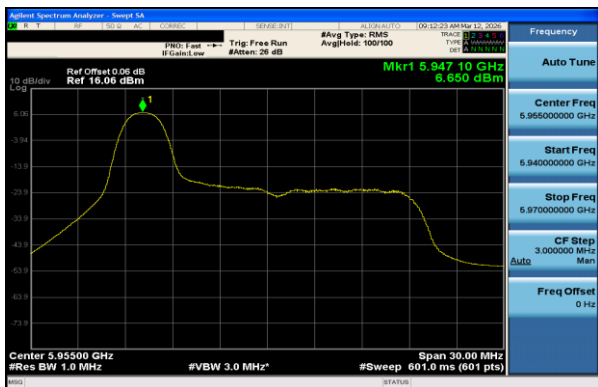
Plot 7-85 PSD Antenna 0 (20MHz BW 802.11ax(RU) RU26 Index0 - Ch.1)
