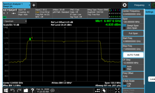
Plot 7-126 PSD Antenna 0 (80MHz BW 802.11ax(RU) RU996 Index67 - Ch.199)
