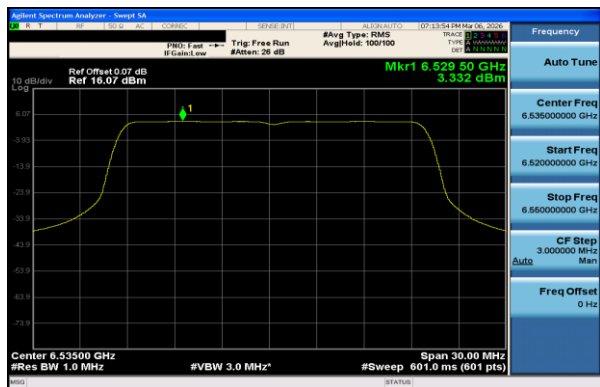
Plot 7-142 PSD Antenna 1 (20MHz BW 802.11ax(RU) RU242 Index61 - Ch.117)
