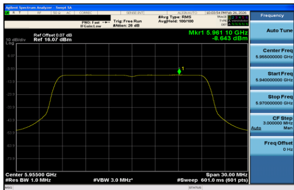
Plot 7-148 PSD Antenna 1 (20MHz BW 802.11ax(RU) RU242 Index61 - Ch.1)
