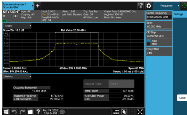
Plot 7-82 26dB BW & 99% OBW Antenna 1 (20MHz BW 802.11ax(RU) RU242 Index61 - Ch.209)
