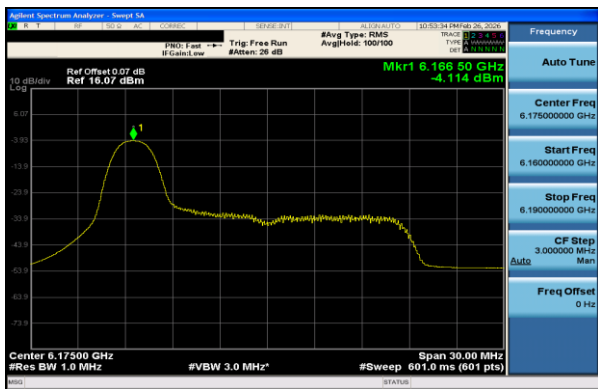
Plot 7-145 PSD Antenna 1 (20MHz BW 802.11ax(RU) RU26 Index0 - Ch.45)
