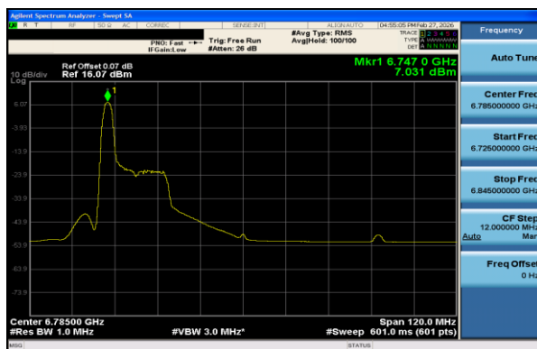
Plot 7-141 PSD Antenna 1 (80MHz BW 802.11ax(RU) RU26 Index0 - Ch.167)
