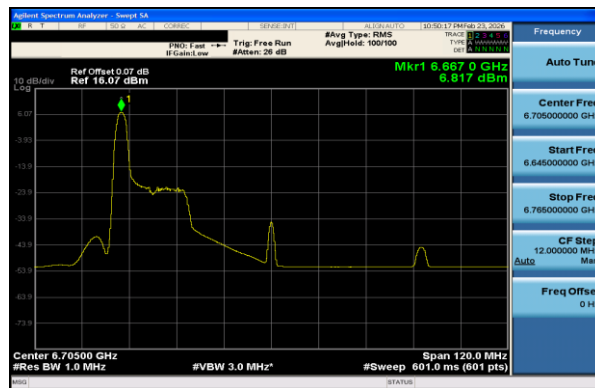
Plot 7-99 PSD Antenna 0 (80MHz BW 802.11ax(RU) RU26 Index0 - Ch.151)
