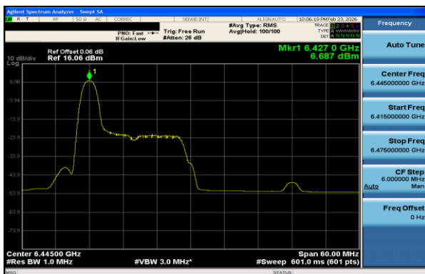
Plot 7-92 PSD Antenna 0 (40MHz BW 802.11ax(RU) RU26 Index0 - Ch.99)
