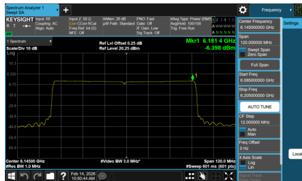
Plot 7-108 PSD Antenna 0 (80MHz BW 802.11ax(RU) RU996 Index67 - Ch.39)
