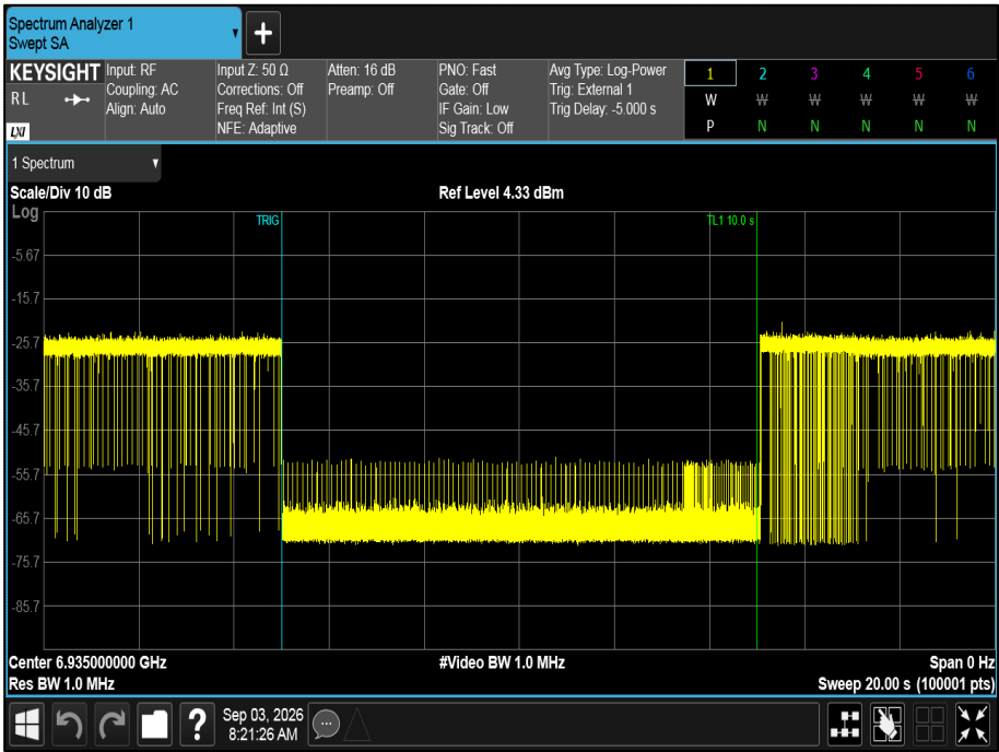
Figure 713 - U-NII-8, Minimum Bandwidth, State: Off
