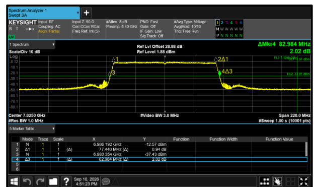
Figure 262 - 802.11ax HE80 SU VLP Maximum 26 dB EBW
