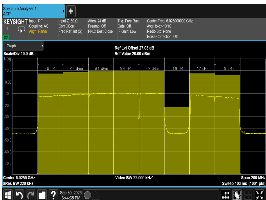
Figure 291 – 6025 MHz (CH 15), 802.11be EHT160 RU996+484+242, MIMO CDD, Adjacent Channel Power
