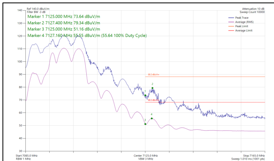
Figure 336 - 802.11be EHT20, RU106+26-83, SDM, Core 0-1 - 7095 MHz Band Edge Frequency 7125 MHz
