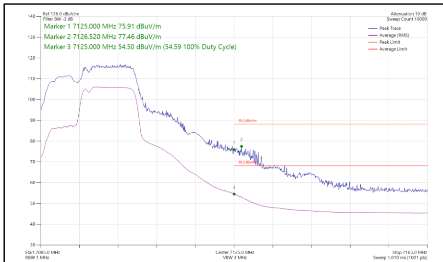
Figure 315 - 802.11be EHT20, RU106+26-83, SISO, Core 1 - 7095 MHz Band Edge Frequency 7125 MHz
