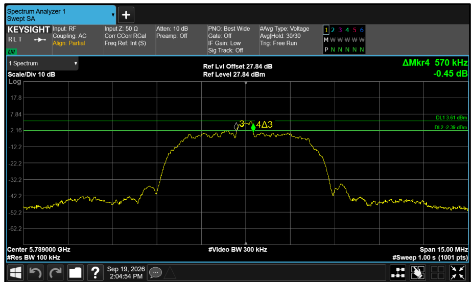
Figure 376 - Core 0 5789 MHz (CH64) 6 dB Bandwidth
