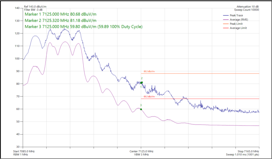
Figure 332 - 802.11be EHT20, RU106+26-83, SDM, Core 0-1 - 7095 MHz Band Edge Frequency 7125 MHz
