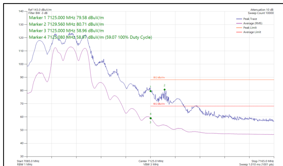
Figure 323 - 802.11be EHT20, RU106+26-83, CDD, Core 0-1 - 7095 MHz Band Edge Frequency 7125 MHz
