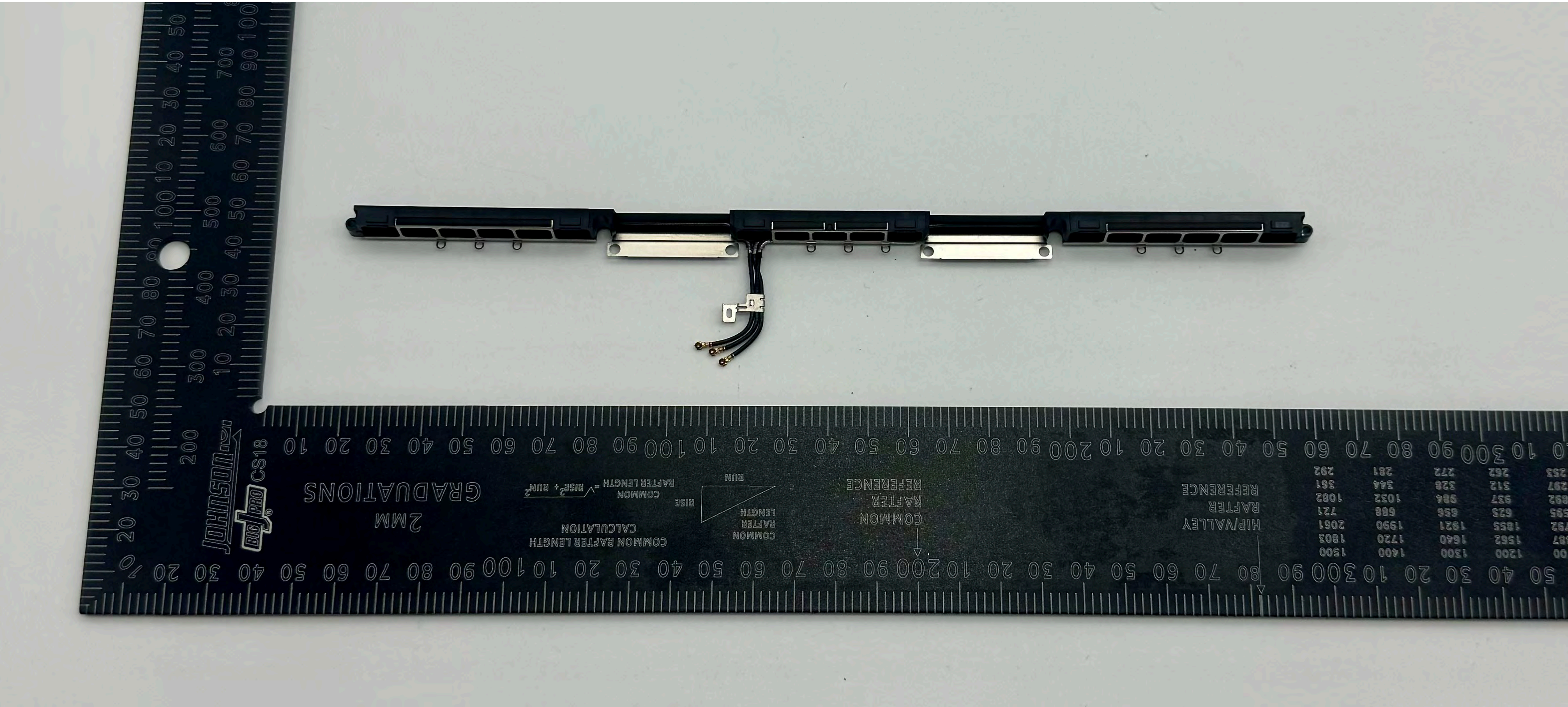
A3401 WF1/BT, WF2/BT, WF3 (BT) antenna structure and feed - Back
