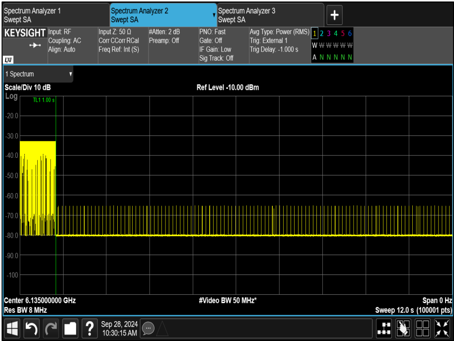
Figure 349 - U-NII-5, Minimum Bandwidth (AWGN High)
