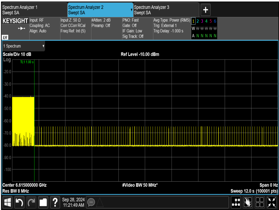
Figure 357 - U-NII-7, Minimum Bandwidth (AWGN High)
