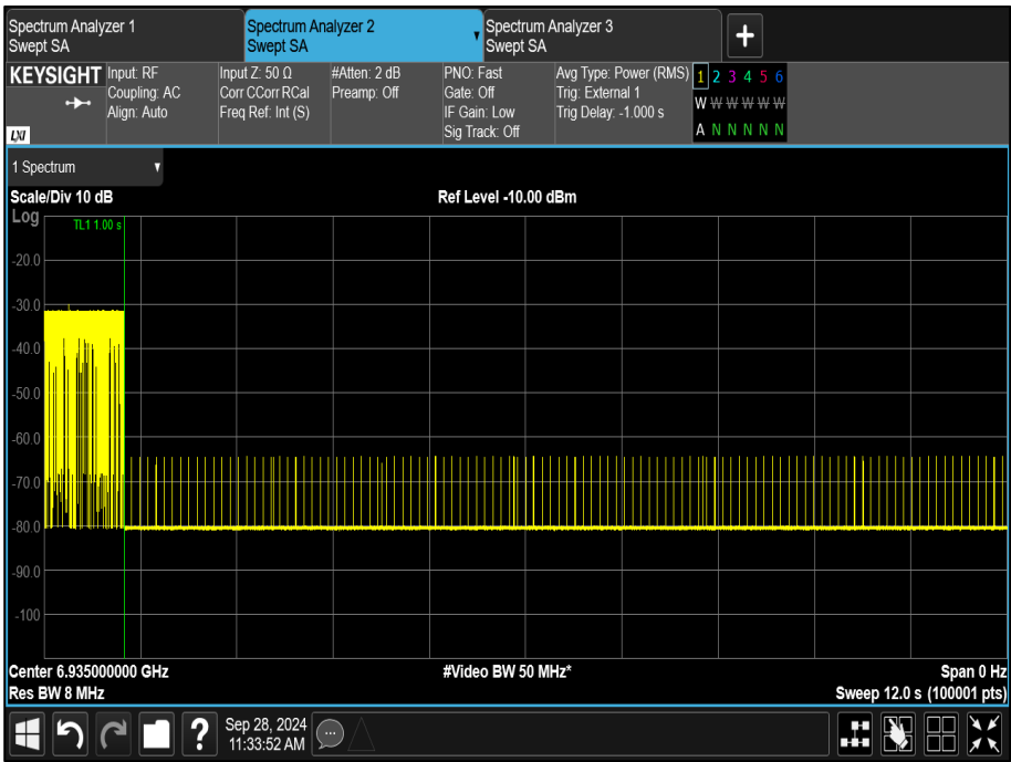
Figure 361 - U-NII-8, Minimum Bandwidth (AWGN High)
