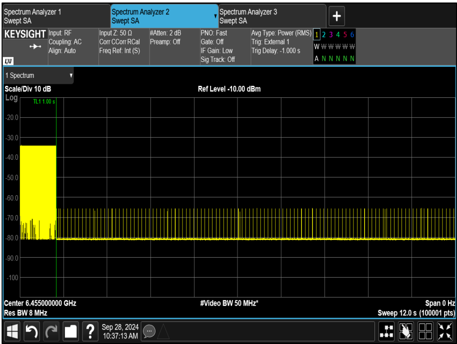
Figure 351 - U-NII-6, Minimum Bandwidth (AWGN Low)
