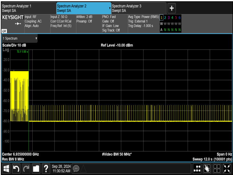
Figure 360 - U-NII-8, Minimum Bandwidth (AWGN Mid)
