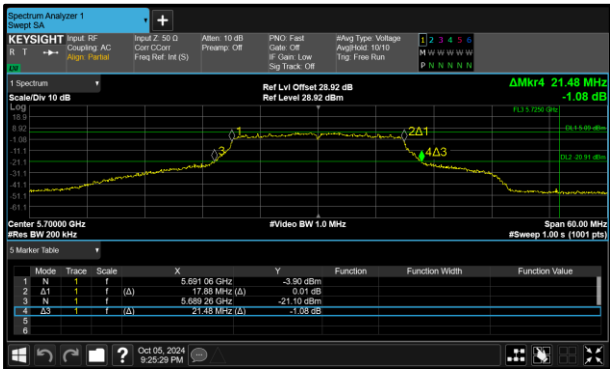
Figure 249 - 802.11ac VHT20 Maximum 99% OBW
