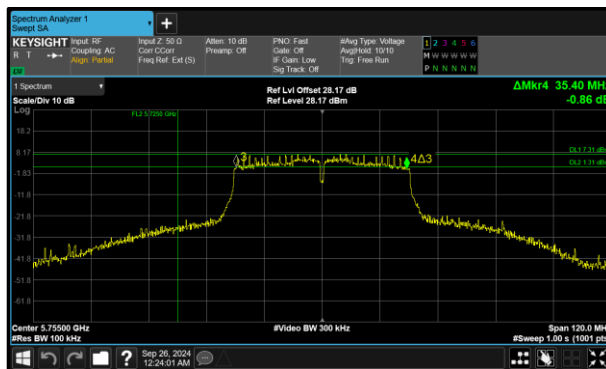
Figure 222 - 802.11n HT40 Minimum 6 dB EBW
