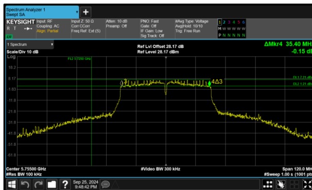
Figure 194 - 802.11n HT40 Minimum 6 dB EBW
