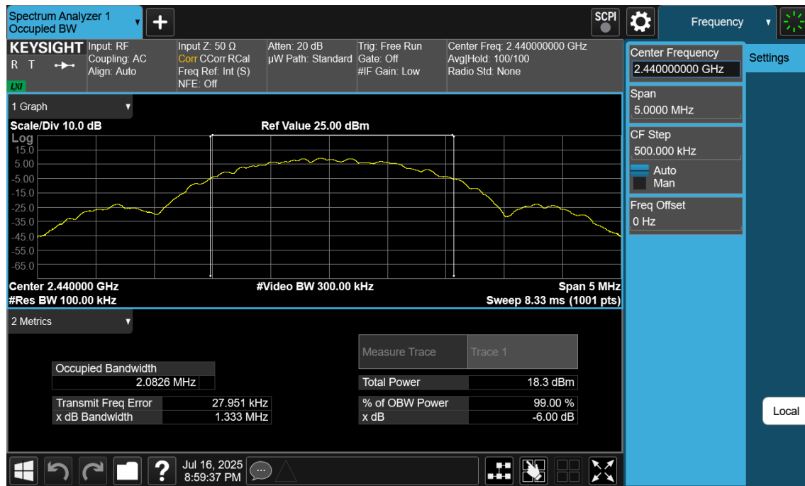
Plot 7-17. 6dB BW & 99% OBW Plot NB UNII_L (Bluetooth (LE), 2Mbps, iPA – Ch. 19)
