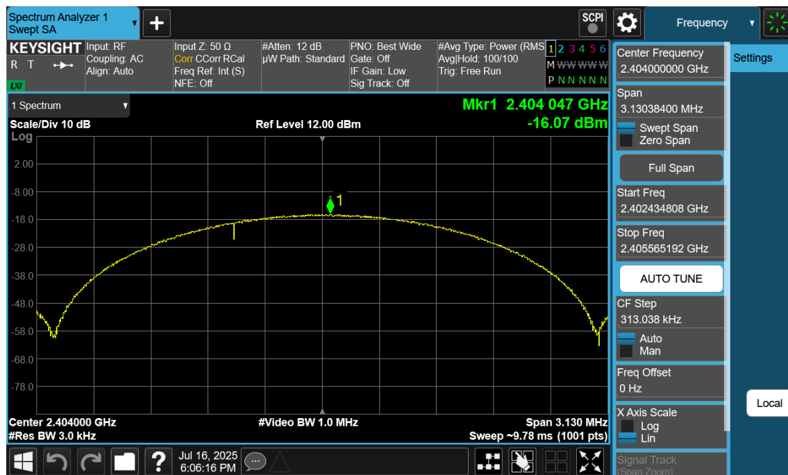
Plot 7-28. Power Spectral Density Plot Ant1 (Bluetooth (LE), 2Mbps, iPA – Ch. 1)
