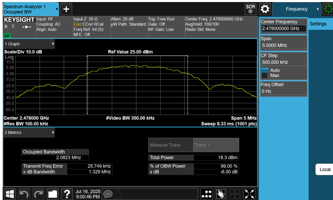
Plot 7-18. 6dB BW & 99% OBW Plot NB UNII_L (Bluetooth (LE), 2Mbps, iPA – Ch. 38)
