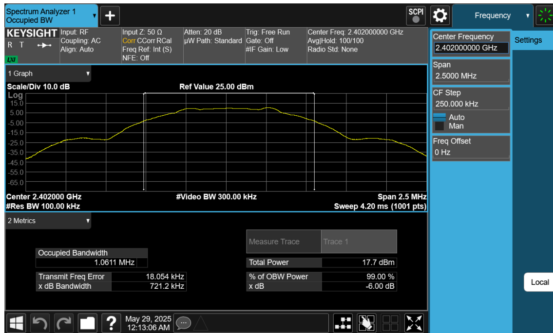
Plot 7-1. 6dB BW & 99% OBW Plot Ant1 (Bluetooth (LE), 1Mbps, ePA – Ch. 0)
