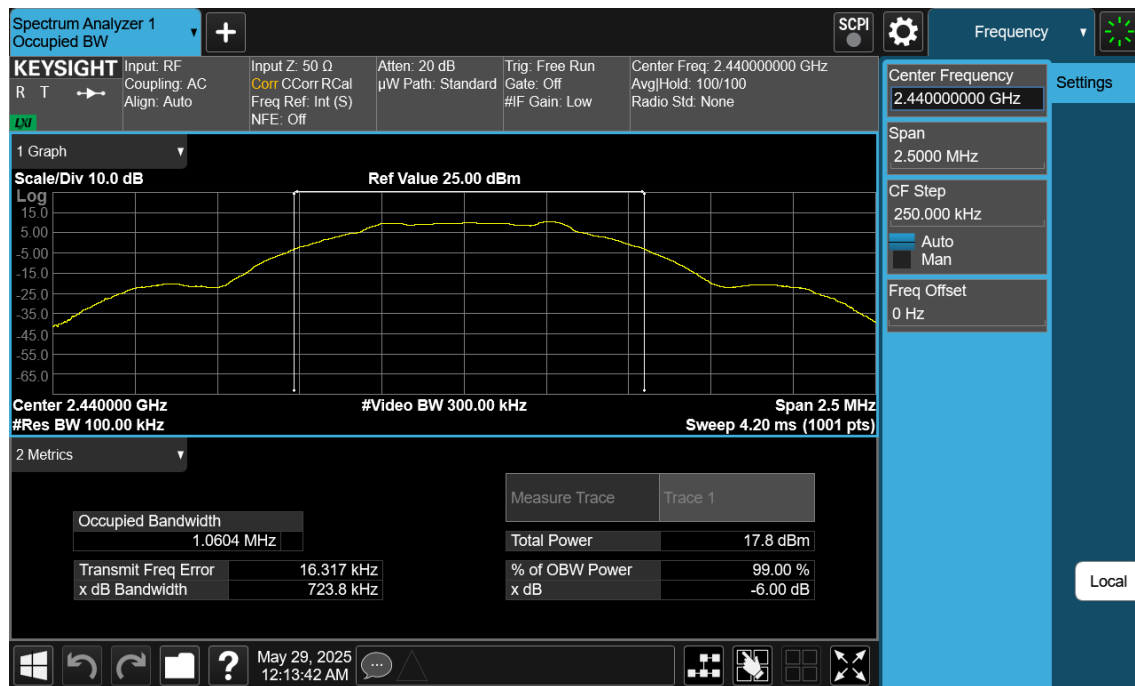
Plot 7-2. 6dB BW & 99% OBW Plot Ant1 (Bluetooth (LE), 1Mbps, ePA – Ch. 19)
