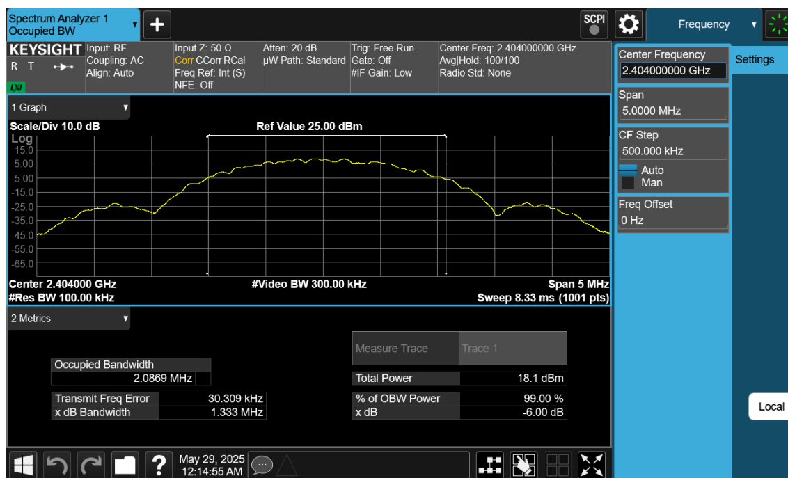
Plot 7-4. 6dB BW & 99% OBW Plot Ant1 (Bluetooth (LE), 2Mbps, ePA – Ch. 1)
