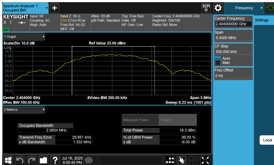
Plot 7-16. 6dB BW & 99% OBW Plot NB UNII_L (Bluetooth (LE), 2Mbps, iPA – Ch. 1)
