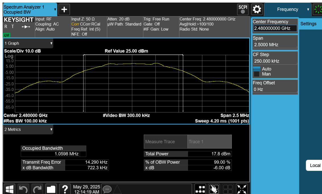
Plot 7-3. 6dB BW & 99% OBW Plot Ant1 (Bluetooth (LE), 1Mbps, ePA – Ch. 39)
