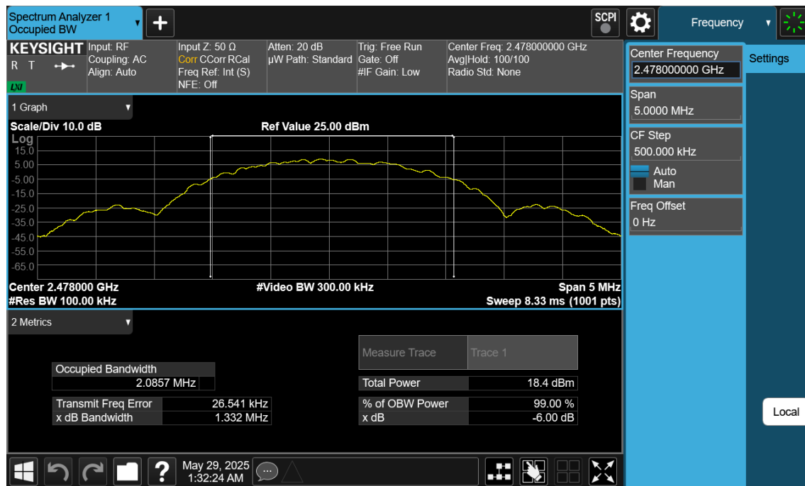
Plot 7-12. 6dB BW & 99% OBW Plot Ant2 (Bluetooth (LE), 2Mbps, ePA – Ch. 38)
