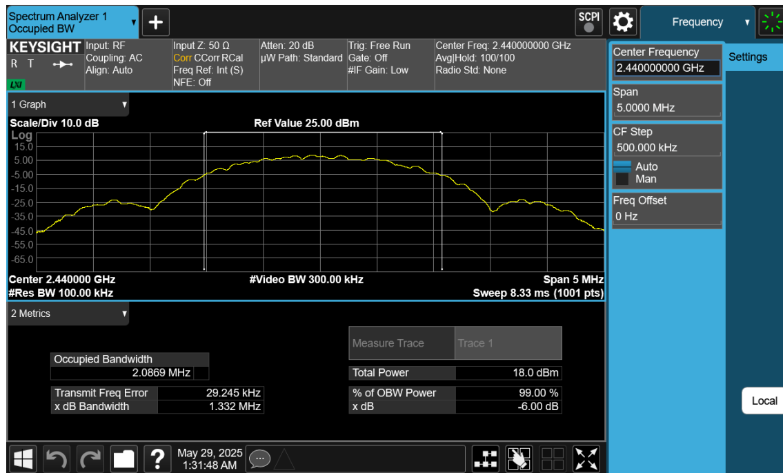
Plot 7-11. 6dB BW & 99% OBW Plot Ant2 (Bluetooth (LE), 2Mbps, ePA – Ch. 19)
