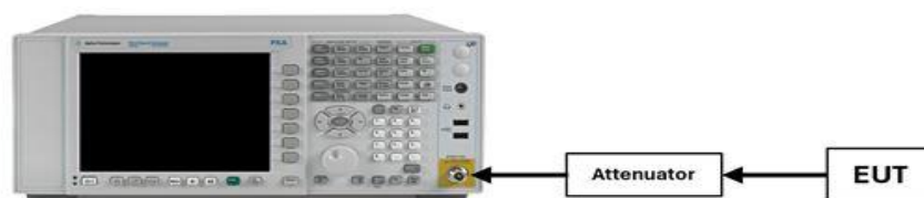
Figure 7-7. Test Instrument & Measurement Setup
