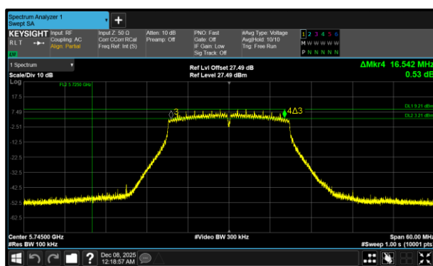
Figure 376 - 802.11a20 Minimum 6 dB EBW
