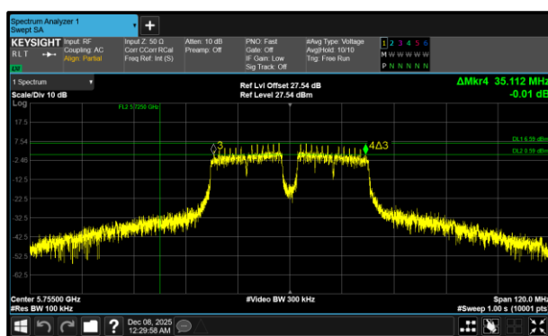
Figure 378 - 802.11a40 Minimum 6 dB EBW
