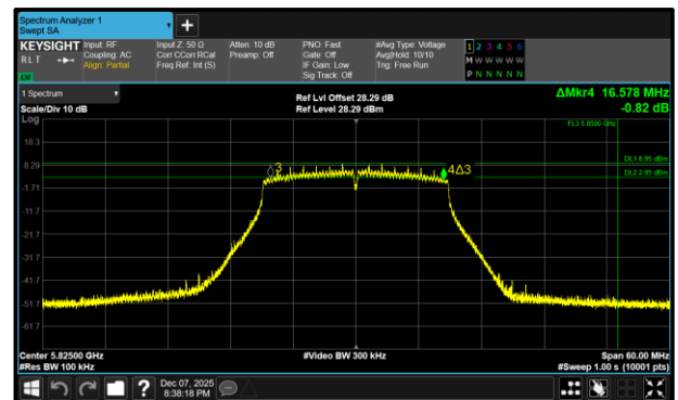
Figure 359 - 802.11a20 Maximum 6 dB EBW
