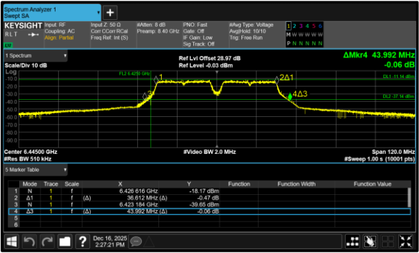
Figure 228 - 802.11a40 VLP Maximum 26 dB EBW
