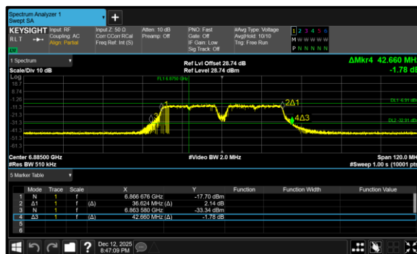
Figure 195 - 802.11a40 LPI Minimum 26 dB EBW
