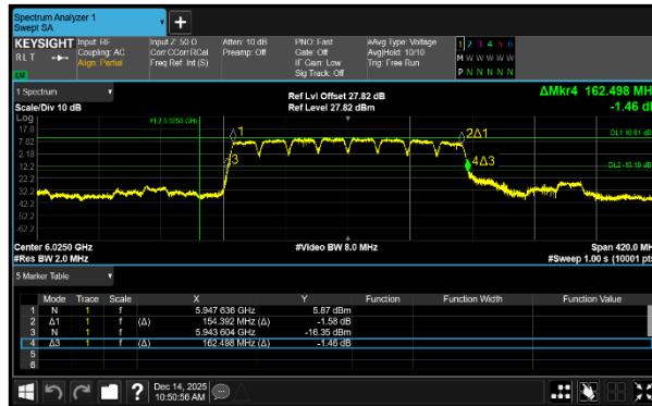
Figure 215 - 802.11a160 SP Minimum 26 dB EBW
