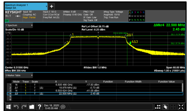
Figure 306 - 802.11ax HE20 SU VLP Maximum 26 dB EBW
