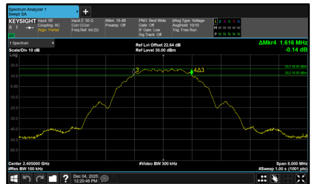
Figure 38 - Core 1 (B) 2405 MHz (CH11) 6 dB Bandwidth
