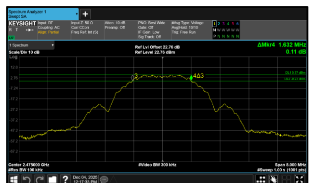
Figure 24 - Core 1 (B) 2475 MHz (CH25) 6 dB Bandwidth
