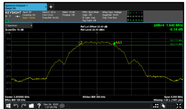
Figure 26 - Core 2 (C) 2405 MHz (CH11) 6 dB Bandwidth
