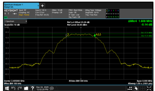
Figure 32 - Core 0 (A) 2405 MHz (CH11) 6 dB Bandwidth
