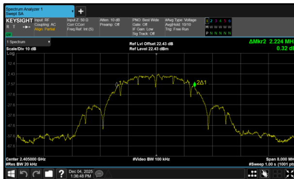
Figure 25 - Core 2 (C) 2405 MHz (CH11) 99% Bandwidth
