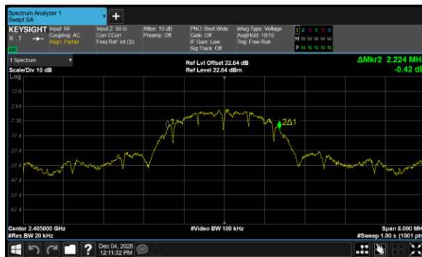
Figure 19 - Core 1 (B) 2405 MHz (CH11) 99% Bandwidth
