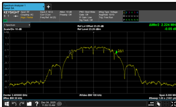
Figure 13 - Core 0 (A) 2405 MHz (CH11) 99% Bandwidth
