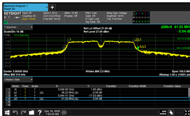
Figure 211 - 802.11a40 SP Minimum 26 dB EBW
