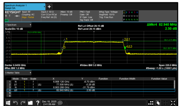
Figure 310 - 802.11ax HE80 SU VLP Maximum 26 dB EBW
