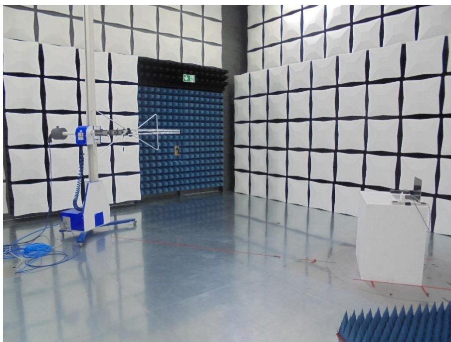
Figure 2 - Radiated Disturbance - Below 1 GHz
