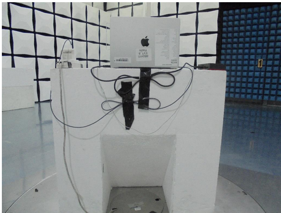
Figure 1 - Radiated Disturbance - Below 1 GHz
