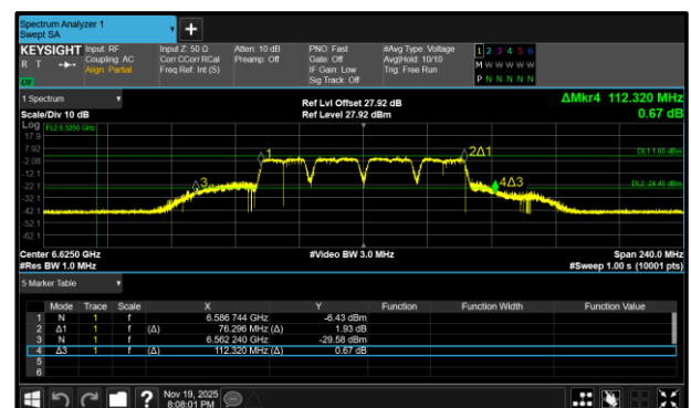
Figure 102 - 802.11a80 LPI Maximum 26 dB EBW
