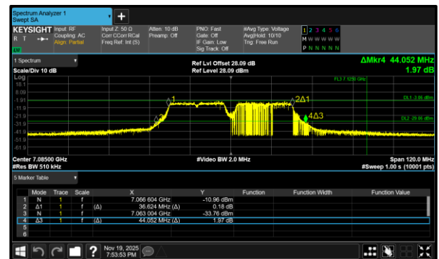
Figure 100 - 802.11a40 LPI Maximum 26 dB EBW
