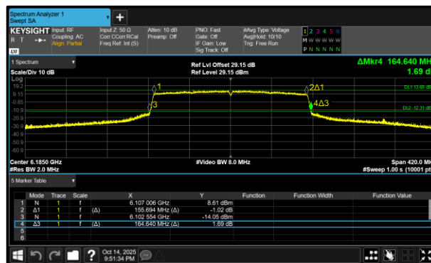
Figure 304 - 802.11ax HE160 SU SP Maximum 26 dB EBW
