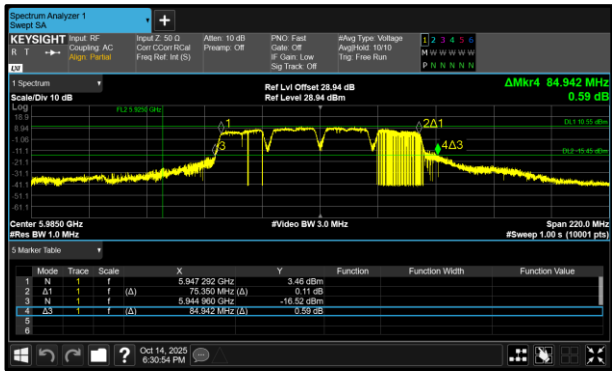
Figure 261 - 802.11a SP (80 MHz) Minimum 99% OBW
