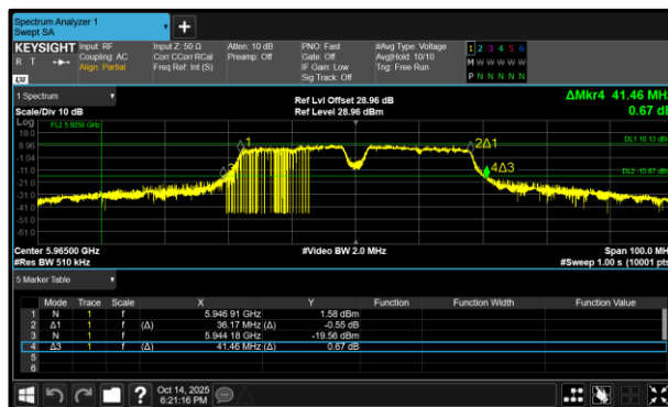
Figure 259 - 802.11a SP (40 MHz) Minimum 99% OBW
