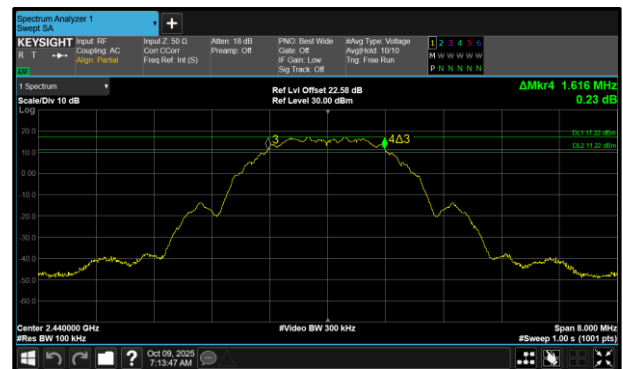
Figure 30 - Core 1 (B) 2440 MHz (CH18) 6 dB Bandwidth
