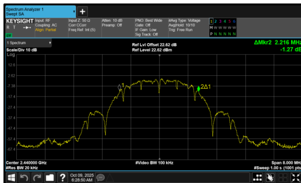
Figure 11 - Core 0 (A) 2440 MHz (CH18) 99% Bandwidth
