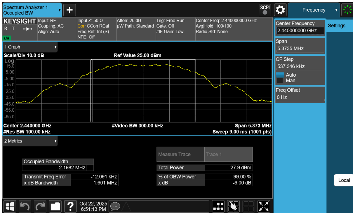
Plot 7-11. 6dB BW Antenna WF7b (802.15.4, Ch. 18)
