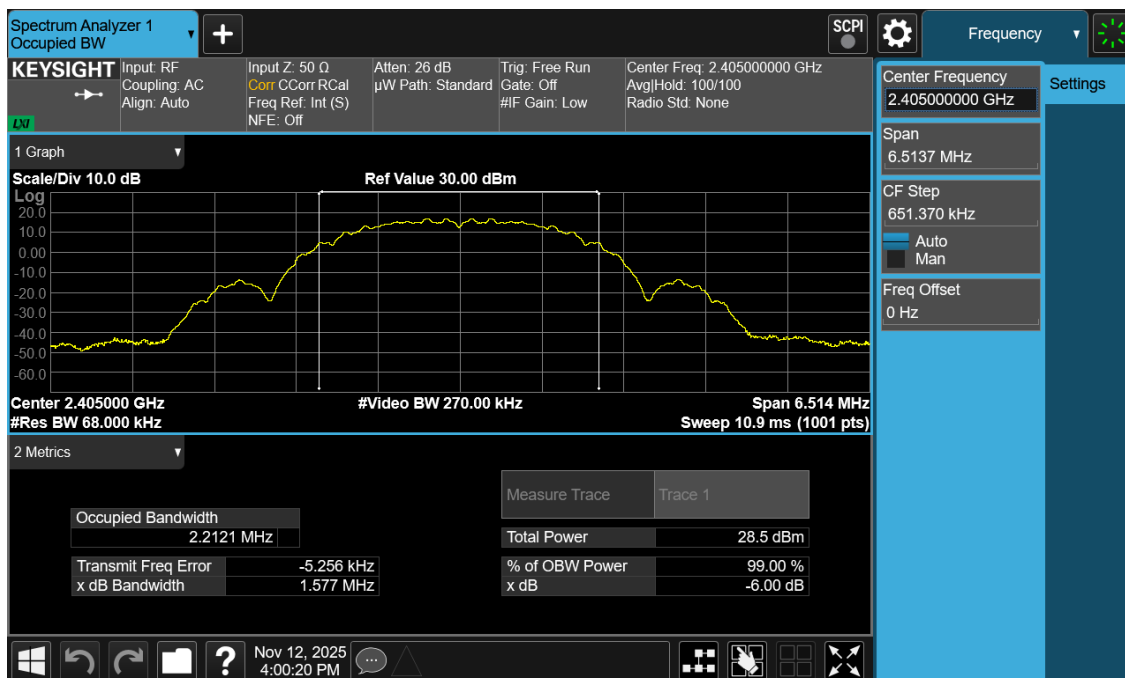
Plot 7-4. 99% OBW Antenna WF7b (802.15.4, Ch. 11)
