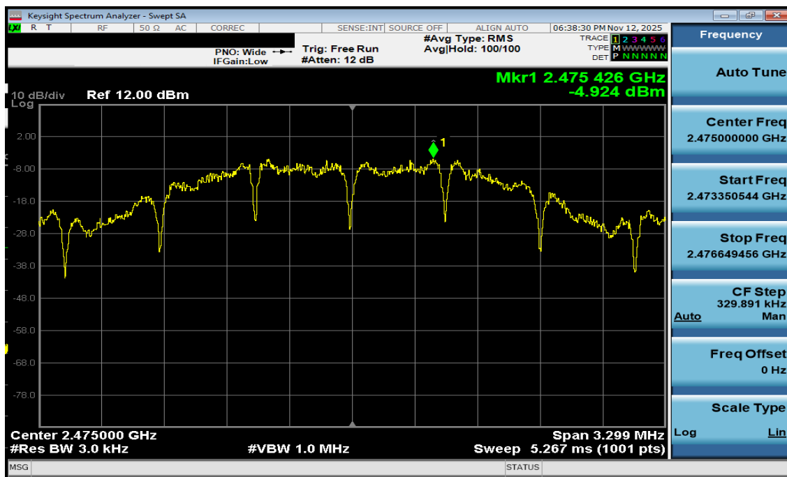
Plot 7-18. Power Spectral Density Antenna WF8 (802.15.4, iPA – Ch. 25)
