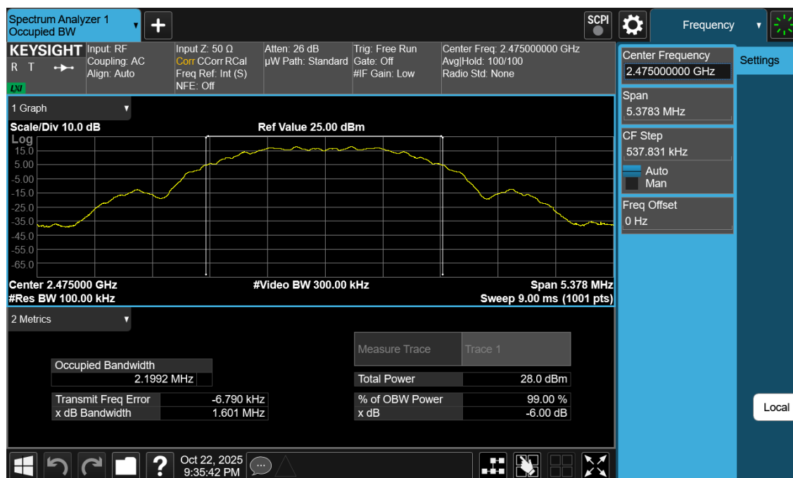
Plot 7-9. 6dB BW Antenna WF8 (802.15.4, Ch. 25)
