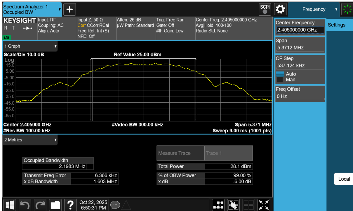
Plot 7-10. 6dB BW Antenna WF7b (802.15.4, Ch. 11)
