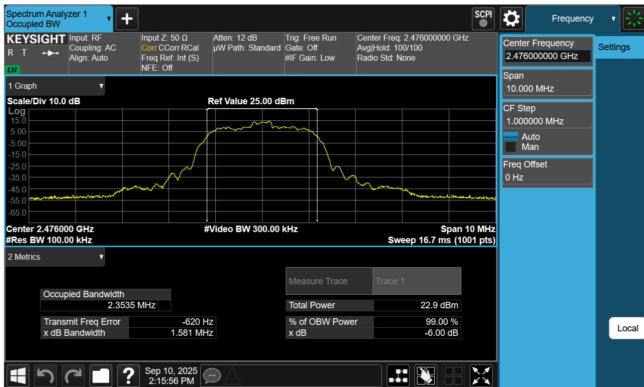
Plot 7-39. 6dB BW Plot Antenna WF8 (Bluetooth (HDR4), 4Mbps, ePA – Ch. 73)
