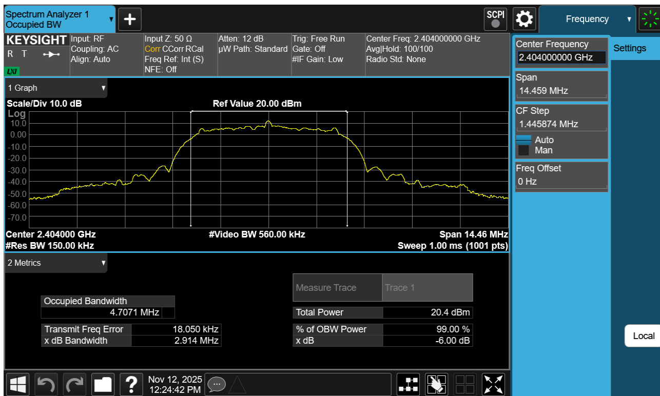
Plot 7-13. 99% OBW Plot Antenna WF8 (Bluetooth (HDRPM16), 16Mbps, ePA – Ch. 1)
