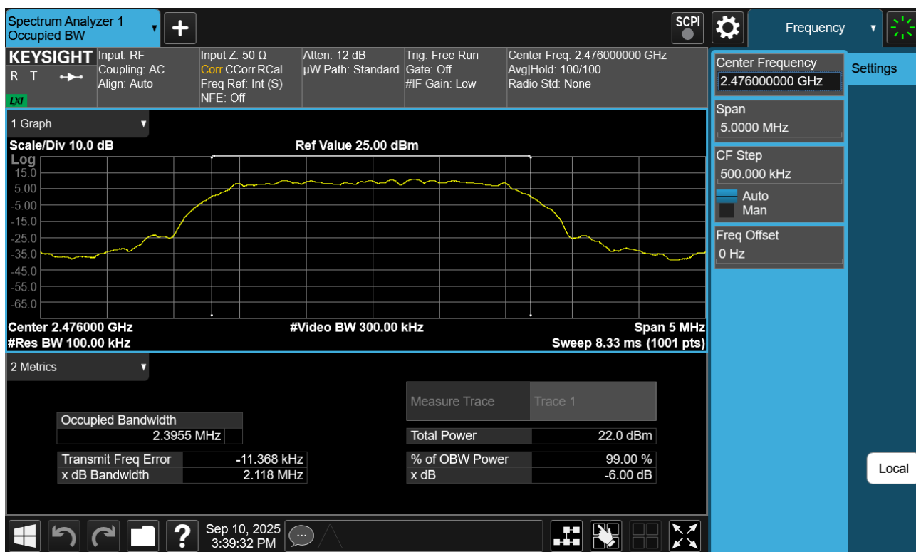
Plot 7-54. 6dB BW Plot Antenna WF8 (Bluetooth (HDT2), 2Mbps, ePA – Ch. 73)
