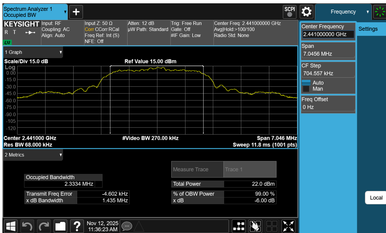
Plot 7-2. 99% OBW Plot Antenna WF8 (Bluetooth (HDR4), 4Mbps, ePA – Ch. 38)
