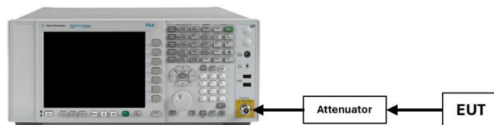
Figure 7-2. Test Instrument & Measurement Setup
