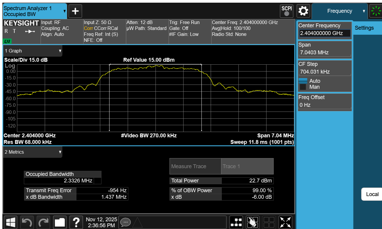
Plot 7-19. 99% OBW Plot Antenna WF7b (Bluetooth (HDR4), 4Mbps, ePA – Ch. 1)
