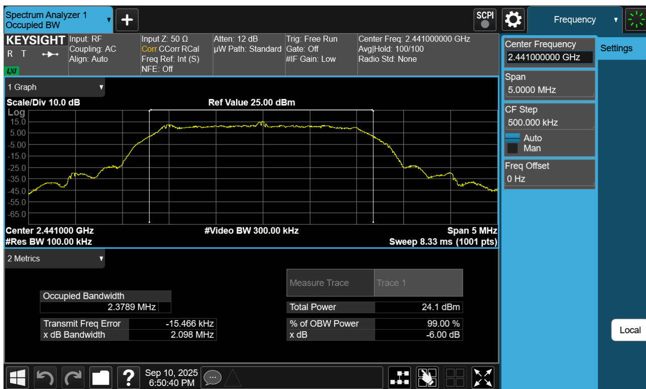
Plot 7-62. 6dB BW Plot Antenna WF7b (Bluetooth (HDRPS2), 2Mbps, ePA – Ch. 38)
