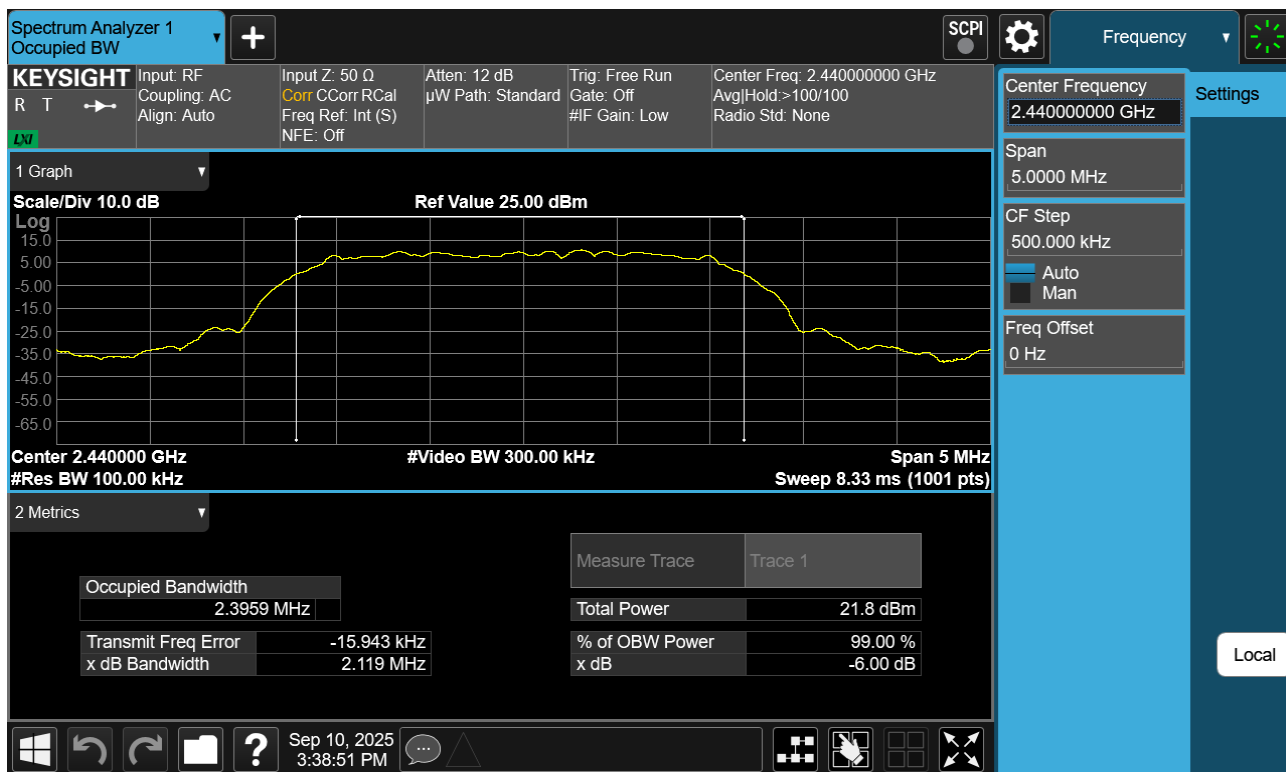
Plot 7-53. 6dB BW Plot Antenna WF8 (Bluetooth (HDT2), 2Mbps, ePA – Ch. 37)
