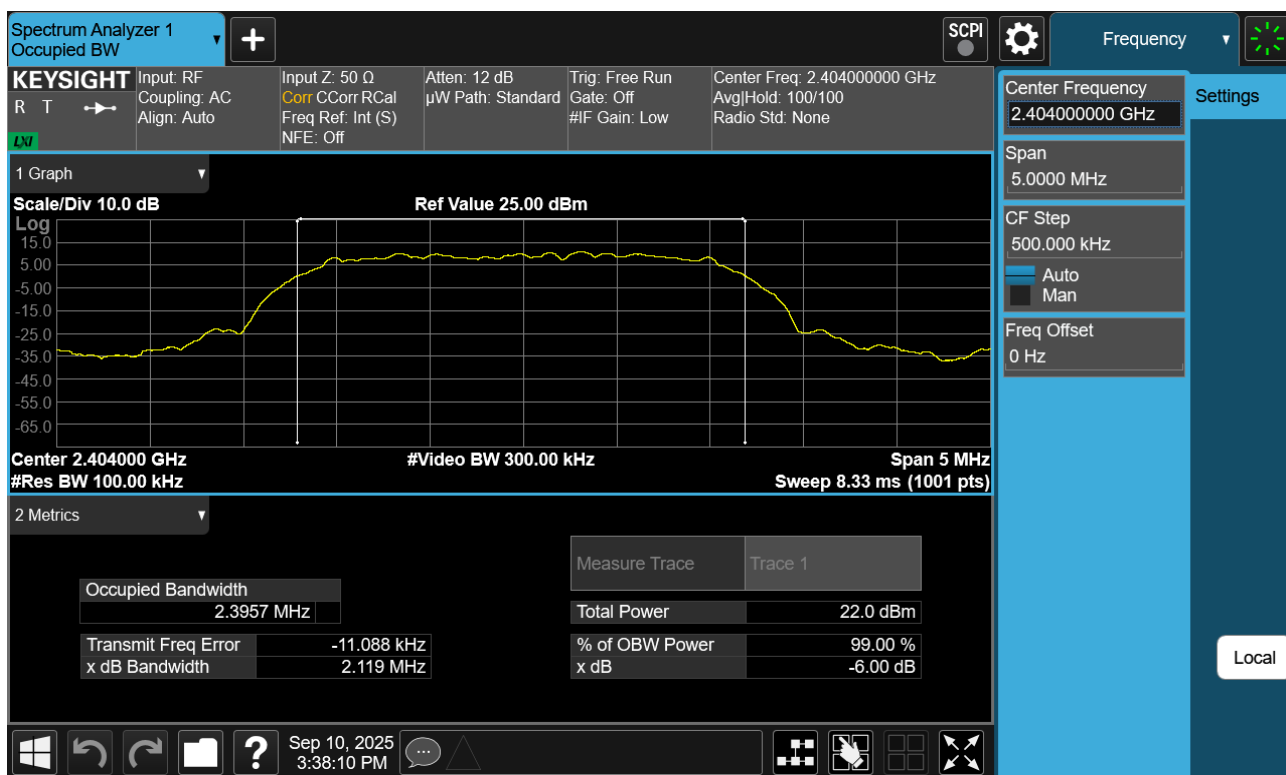
Plot 7-52. 6dB BW Plot Antenna WF8 (Bluetooth (HDT2), 2Mbps, ePA – Ch. 1)
