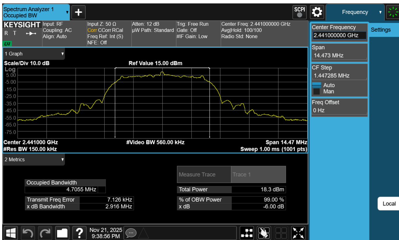
Plot 7-14. 99% OBW Plot Antenna WF8 (Bluetooth (HDRPM16), 16Mbps, ePA – Ch. 38)
