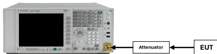
Figure 7-1. Test Instrument & Measurement Setup
