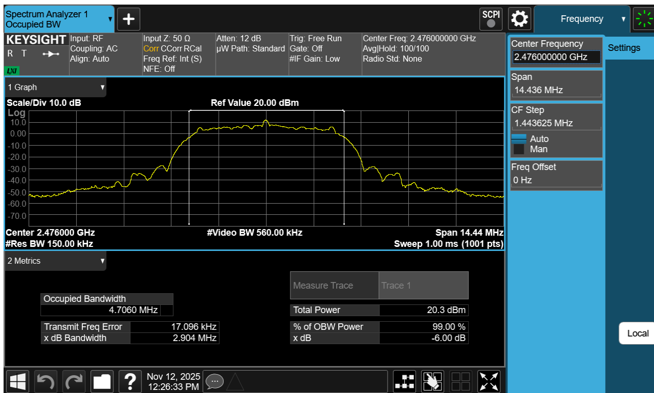
Plot 7-15. 99% OBW Plot Antenna WF8 (Bluetooth (HDRPM16), 16Mbps, ePA – Ch. 73)
