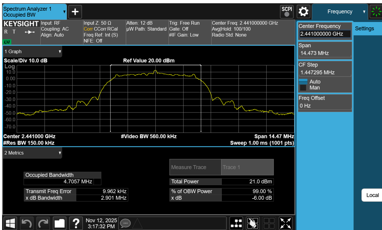
Plot 7-32. 99% OBW Plot Antenna WF7b (Bluetooth (HDRPM16), 16Mbps, ePA – Ch. 38)
