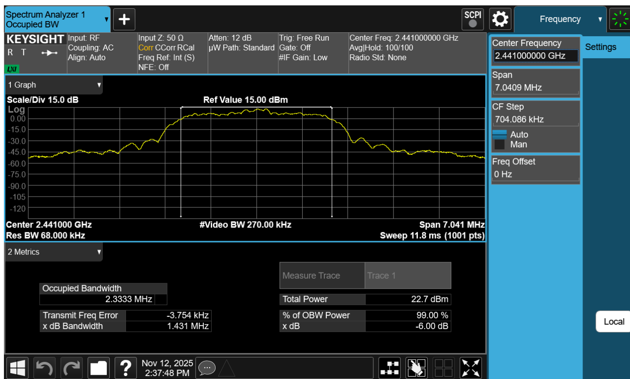
Plot 7-20. 99% OBW Plot Antenna WF7b (Bluetooth (HDR4), 4Mbps, ePA – Ch. 38)
