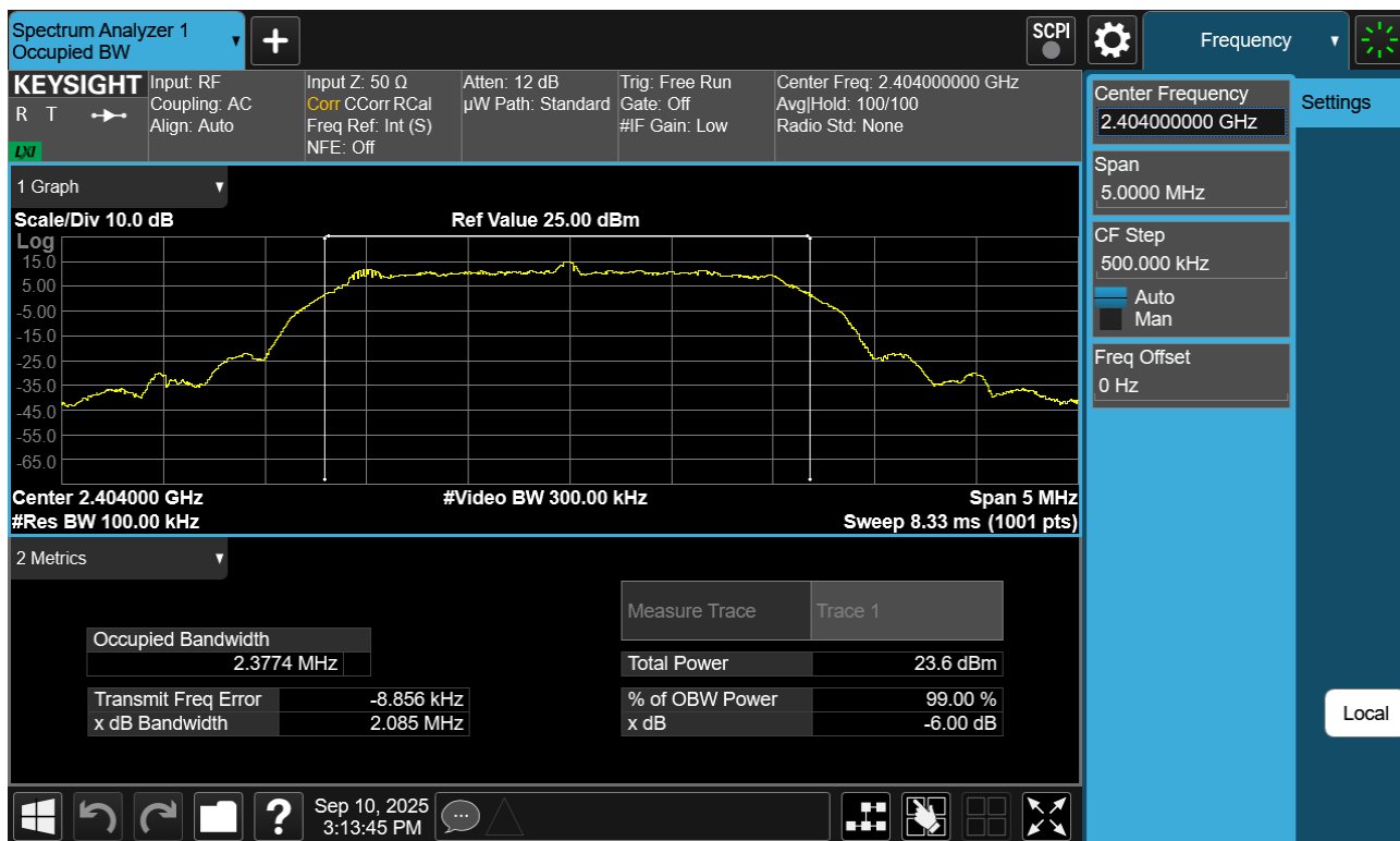
Plot 7-43. 6dB BW Plot Antenna WF8 (Bluetooth (HDRPS2), 2Mbps, ePA – Ch. 1)
