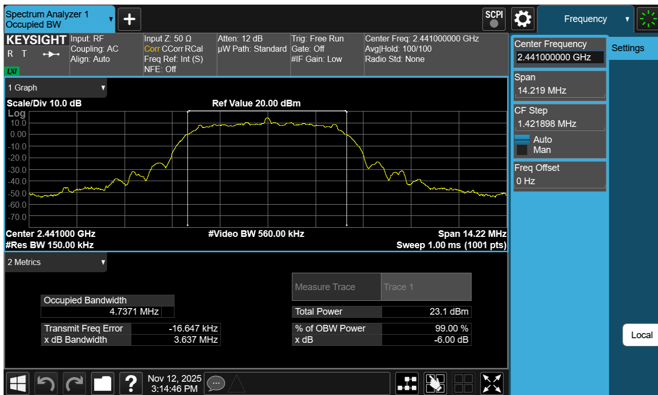
Plot 7-29. 99% OBW Plot Antenna WF7b (Bluetooth (XHDRPM6), 6Mbps, ePA – Ch. 38)
