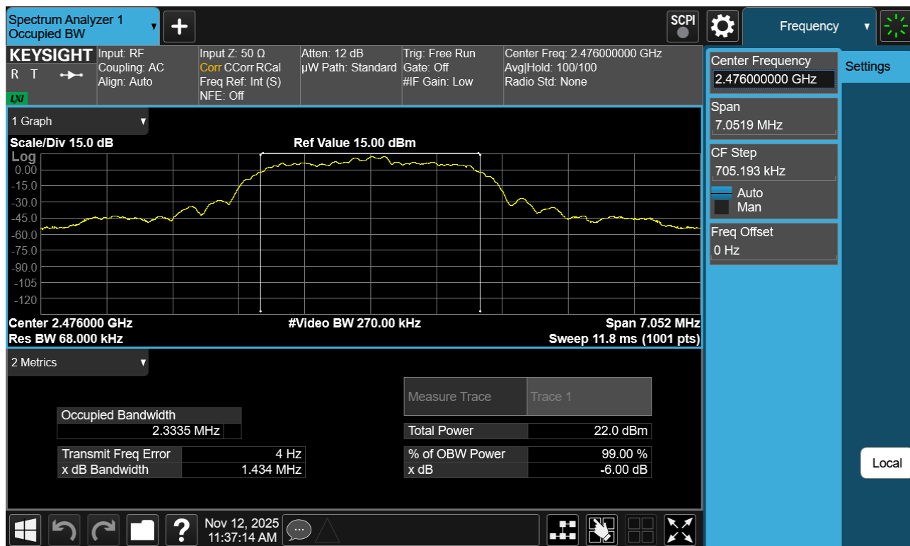
Plot 7-3. 99% OBW Plot Antenna WF8 (Bluetooth (HDR4), 4Mbps, ePA – Ch. 73)
