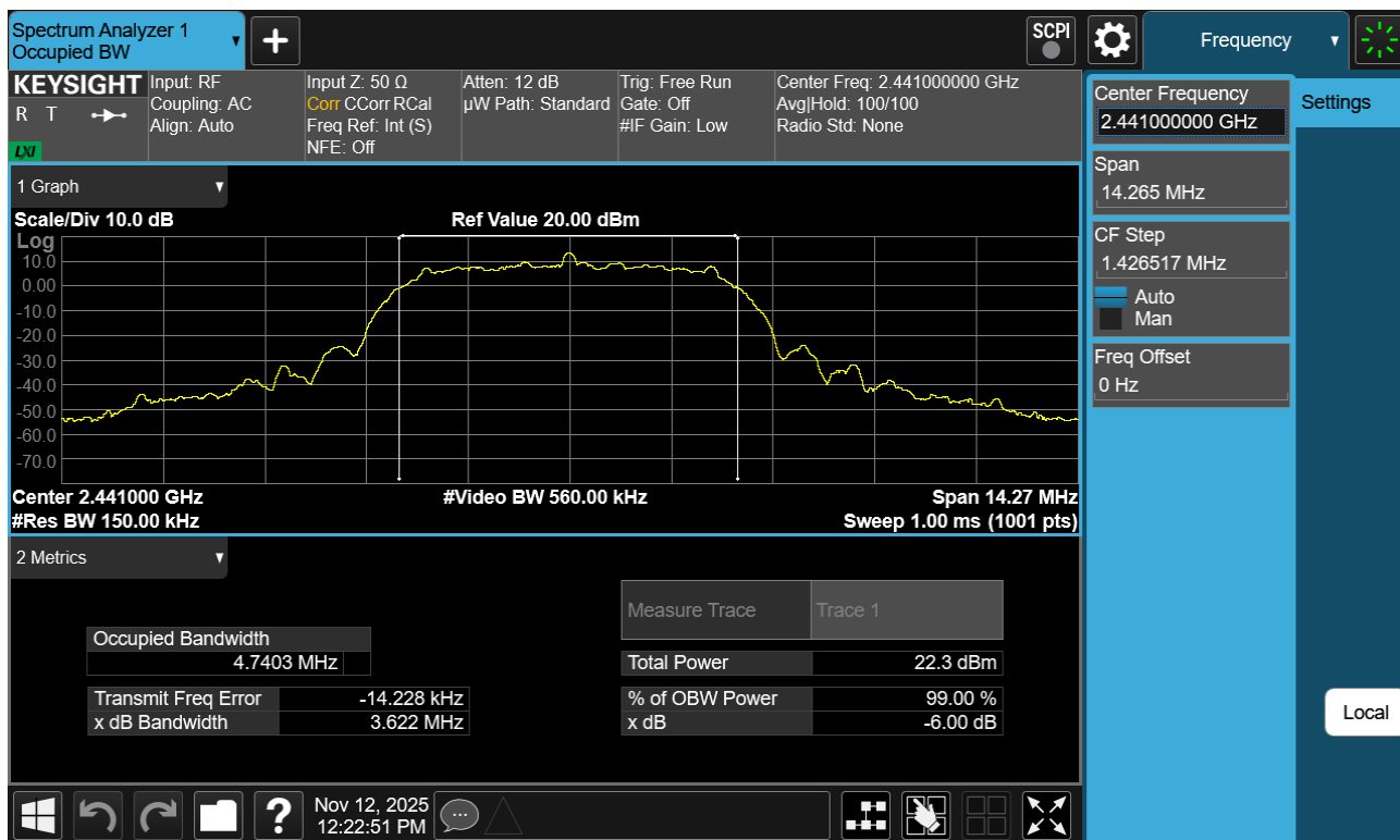
Plot 7-11. 99% OBW Plot Antenna WF8 (Bluetooth (XHDRPM6), 6Mbps, ePA – Ch. 38)
