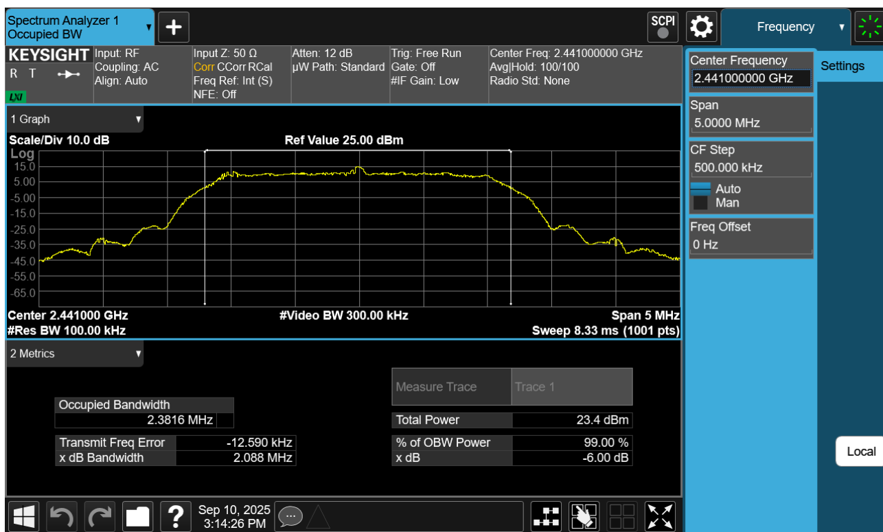
Plot 7-44. 6dB BW Plot Antenna WF8 (Bluetooth (HDRPS2), 2Mbps, ePA – Ch. 38)
