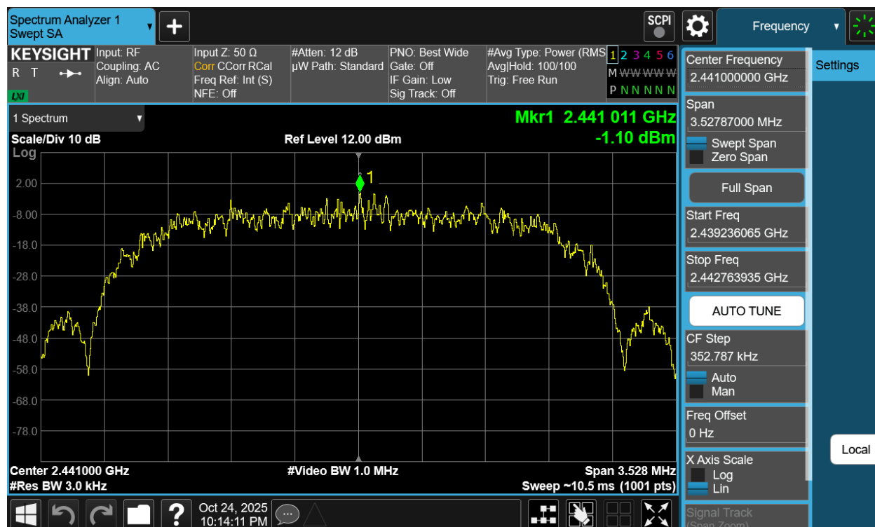
Plot 7-110. Power Spectral Density Plot Antenna WF7b (Bluetooth (HDR4), 4Mbps, ePA – Ch. 38)
