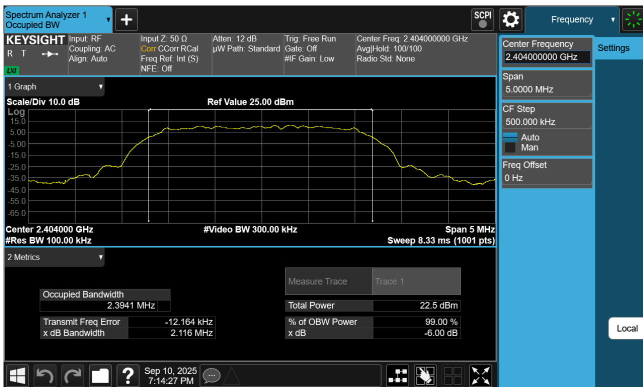
Plot 7-70. 6dB BW Plot Antenna WF7b (Bluetooth (HDT2), 2Mbps, ePA – Ch. 1)
