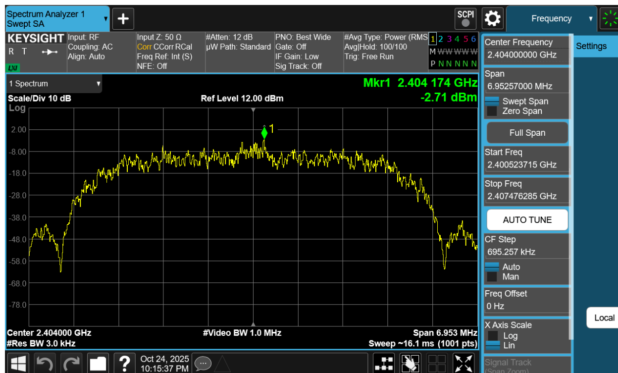
Plot 7-115. Power Spectral Density Plot Antenna WF7b (Bluetooth (HDR8), 8Mbps, ePA – Ch. 1)
