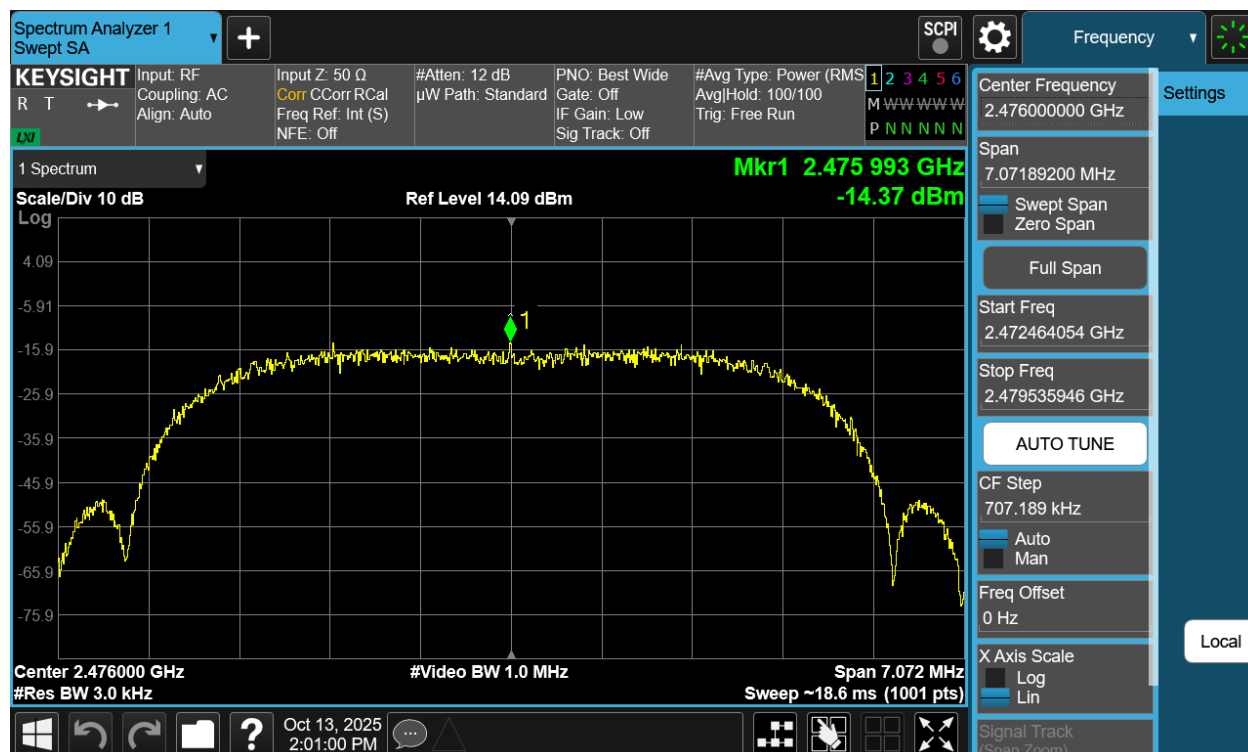
Plot 7-96. Power Spectral Density Plot Antenna WF8 (Bluetooth (XHDRPM6), 6Mbps, iPA – Ch. 73)
