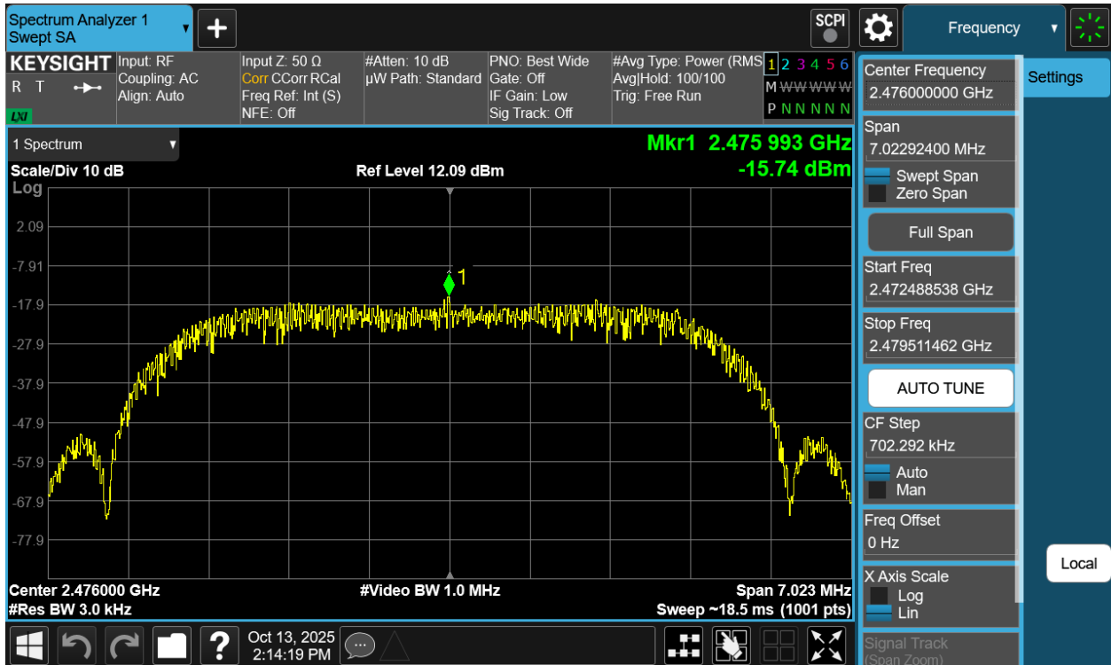
Plot 7-102. Power Spectral Density Plot Antenna WF8 (Bluetooth (HDRPM16), 16Mbps, iPA – Ch. 73)
