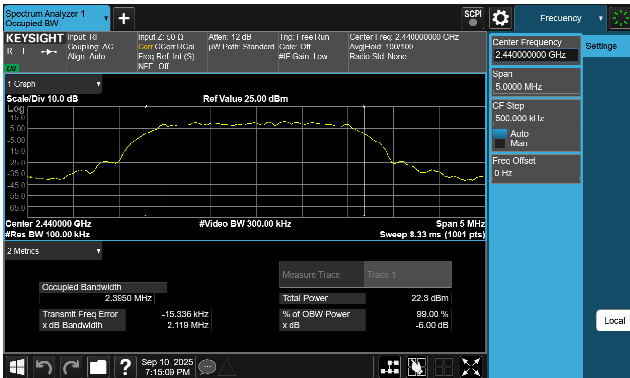
Plot 7-71. 6dB BW Plot Antenna WF7b (Bluetooth (HDT2), 2Mbps, ePA – Ch. 37)
