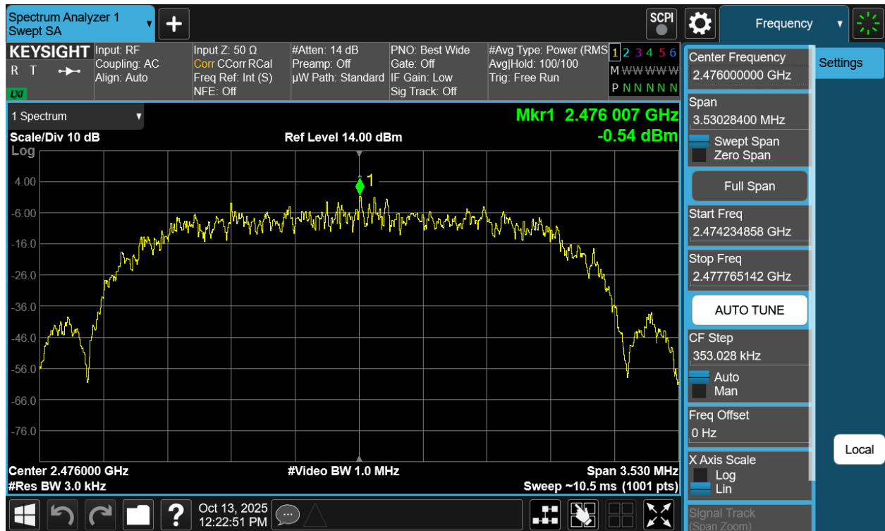
Plot 7-75. Power Spectral Density Plot Antenna WF8 (Bluetooth (HDR4), 4Mbps, ePA – Ch. 73)
