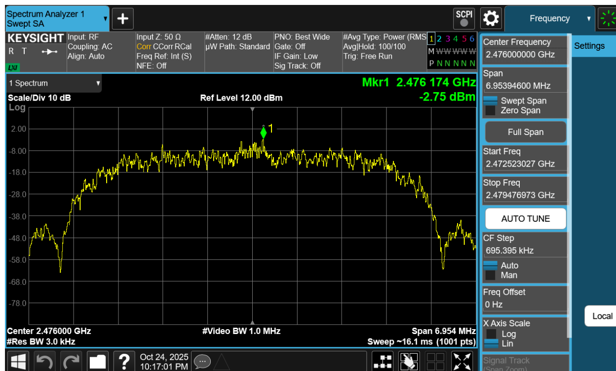
Plot 7-117. Power Spectral Density Plot Antenna WF7b (Bluetooth (HDR8), 8Mbps, ePA – Ch. 73)
