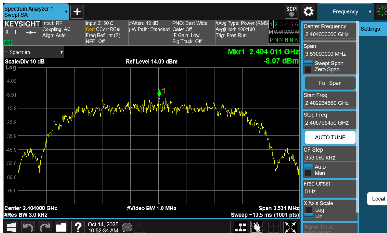
Plot 7-112. Power Spectral Density Plot Antenna WF7b (Bluetooth (HDR4), 4Mbps, iPA – Ch. 1)
