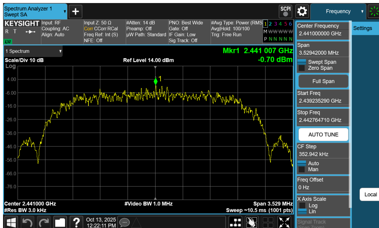
Plot 7-74. Power Spectral Density Plot Antenna WF8 (Bluetooth (HDR4), 4Mbps, ePA – Ch. 38)
