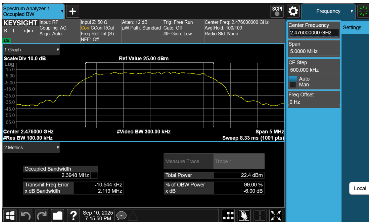
Plot 7-72. 6dB BW Plot Antenna WF7b (Bluetooth (HDT2), 2Mbps, ePA – Ch. 73)
