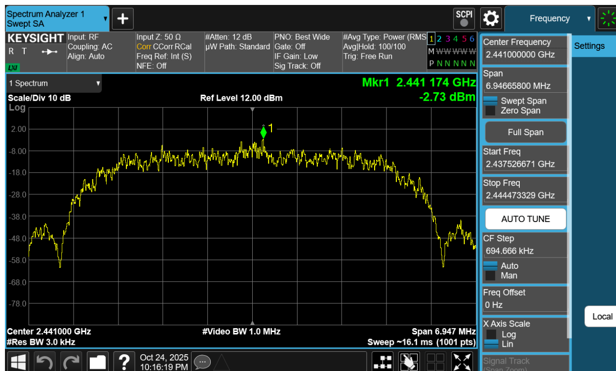
Plot 7-116. Power Spectral Density Plot Antenna WF7b (Bluetooth (HDR8), 8Mbps, ePA – Ch. 38)
