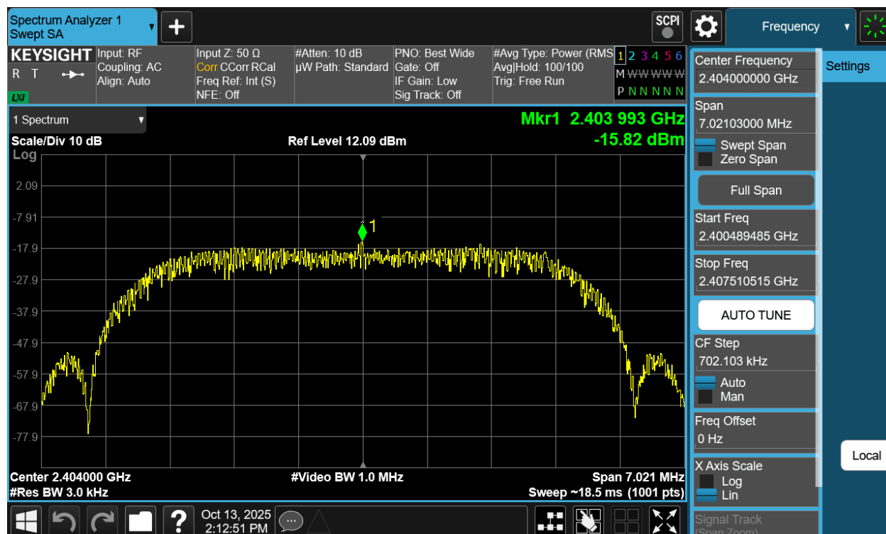
Plot 7-100. Power Spectral Density Plot Antenna WF8 (Bluetooth (HDRPM16), 16Mbps, iPA – Ch. 1)
