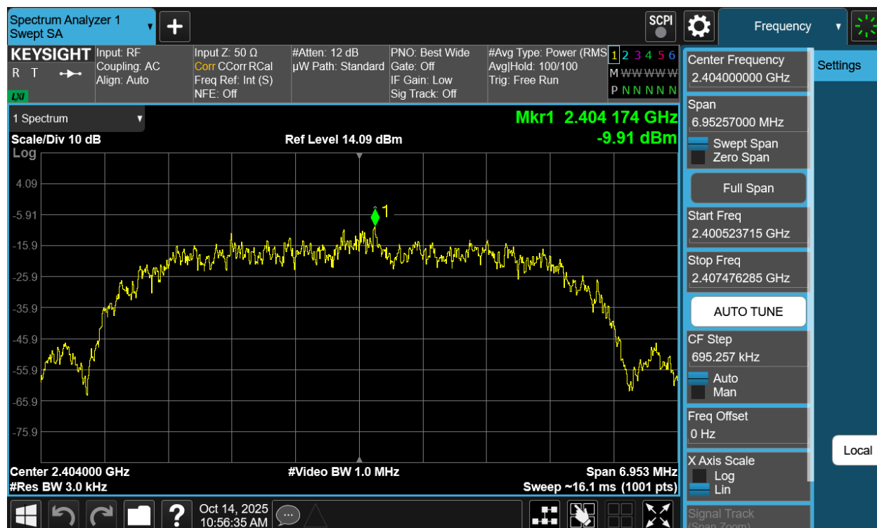
Plot 7-118. Power Spectral Density Plot Antenna WF7b (Bluetooth (HDR8), 8Mbps, iPA – Ch. 1)
