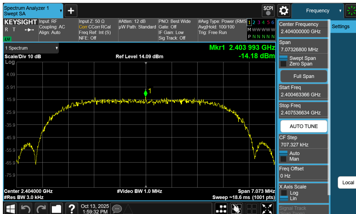
Plot 7-94. Power Spectral Density Plot Antenna WF8 (Bluetooth (XHDRPM6), 6Mbps, iPA – Ch. 1)
