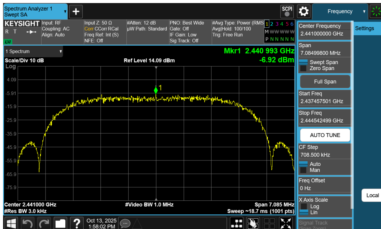
Plot 7-92. Power Spectral Density Plot Antenna WF8 (Bluetooth (XHDRPM6), 6Mbps, ePA – Ch. 38)
