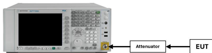
Figure 7-2. Test Instrument & Measurement Setup
