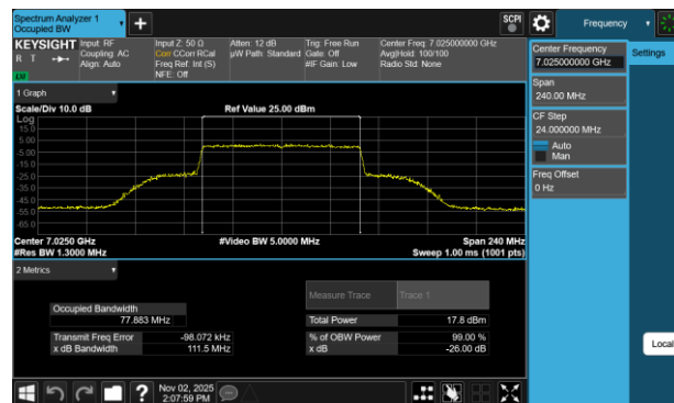
Plot 7-15 26dB BW & 99% OBW Antenna WF8 (80MHz BW 802.11be(SU) - Ch.215)
