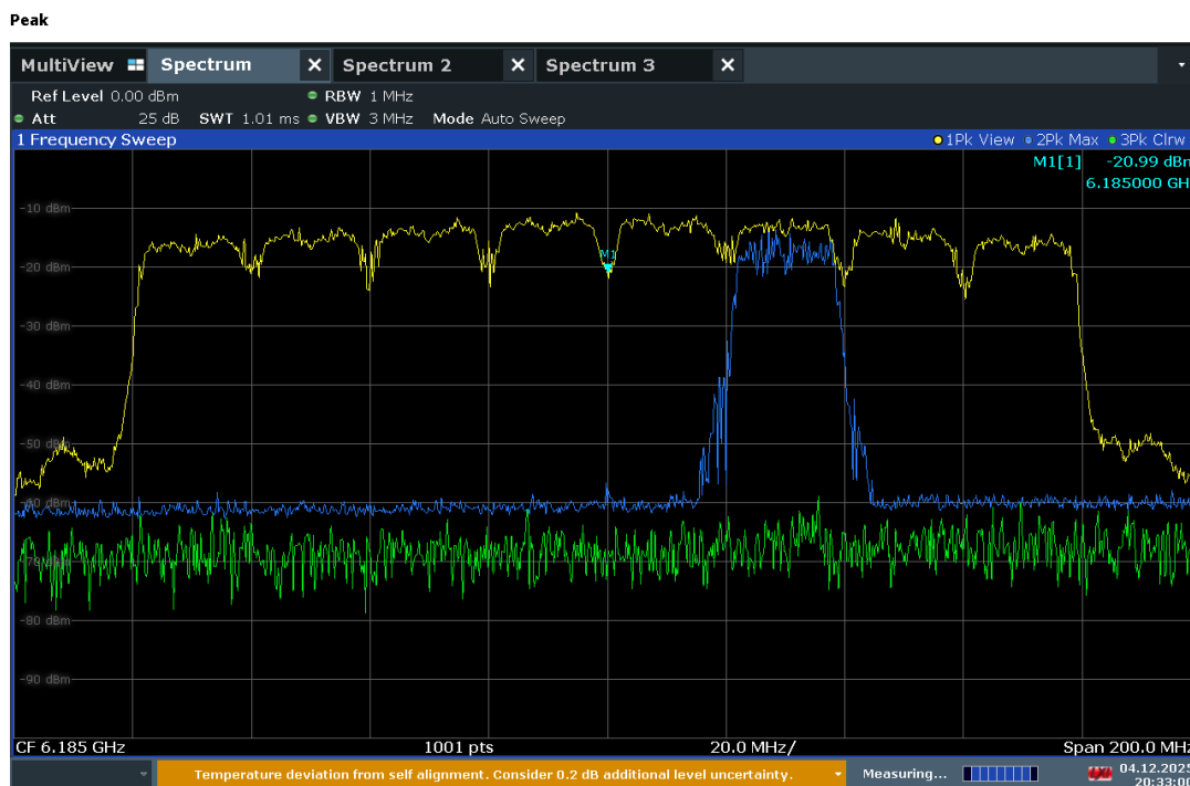
Plot 7-210. 160MHz Bandwidth, AWGN Signal Injected – 6185MHz
