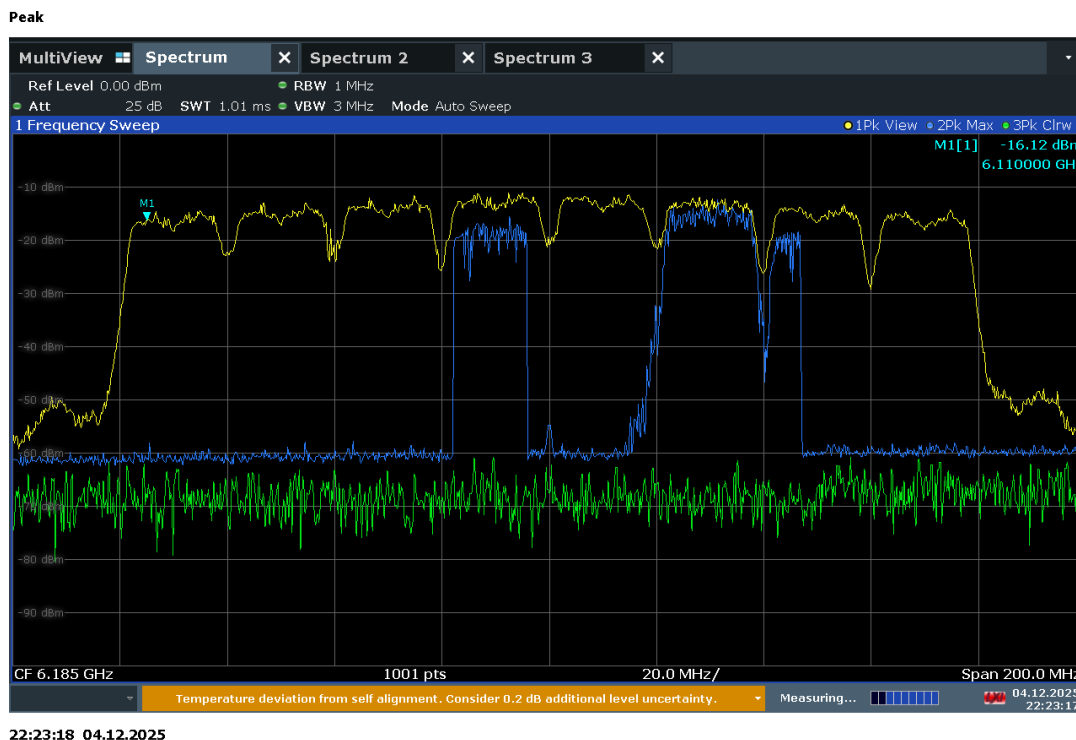
Plot 7-209. 160MHz Bandwidth, AWGN Signal Injected – 6110Mhz
