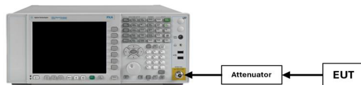
Figure 7-3. Test Instrument & Measurement Setup
