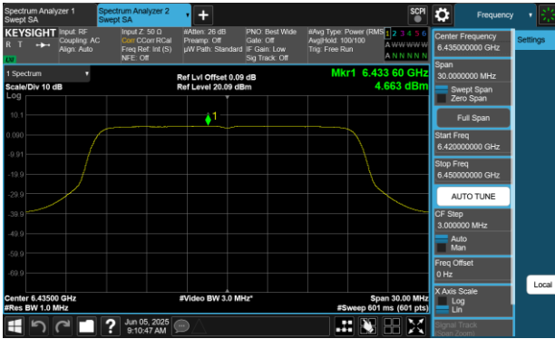
Plot 7-345 PSD CDD Antenna WF8 (20MHz BW 802.11be(RU) RU242 Index61 - Ch.97)
