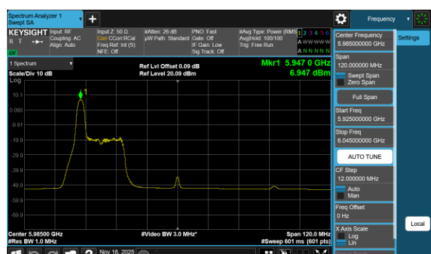
Plot 7-315 PSD SDM Antenna WF7a (80MHz BW 802.11be(RU) RU26 Index0 - Ch.7)
