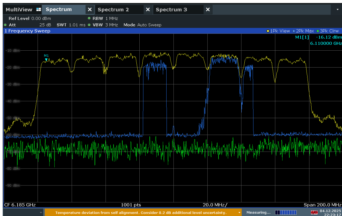
Plot 7-489. 160MHz Bandwidth, AWGN Signal Injected – 6110MHz
