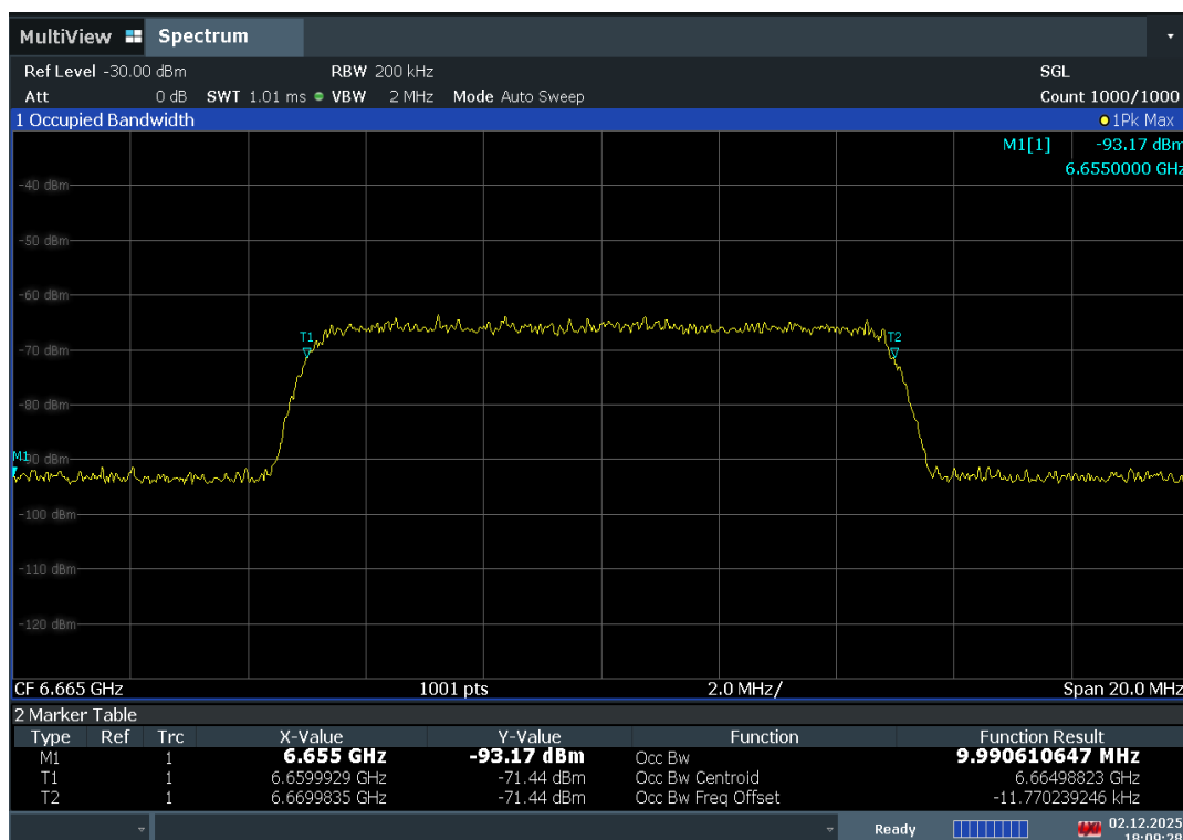
Plot 7-451. AWGN Signal – UNII 7 – 160MHz – Mid
