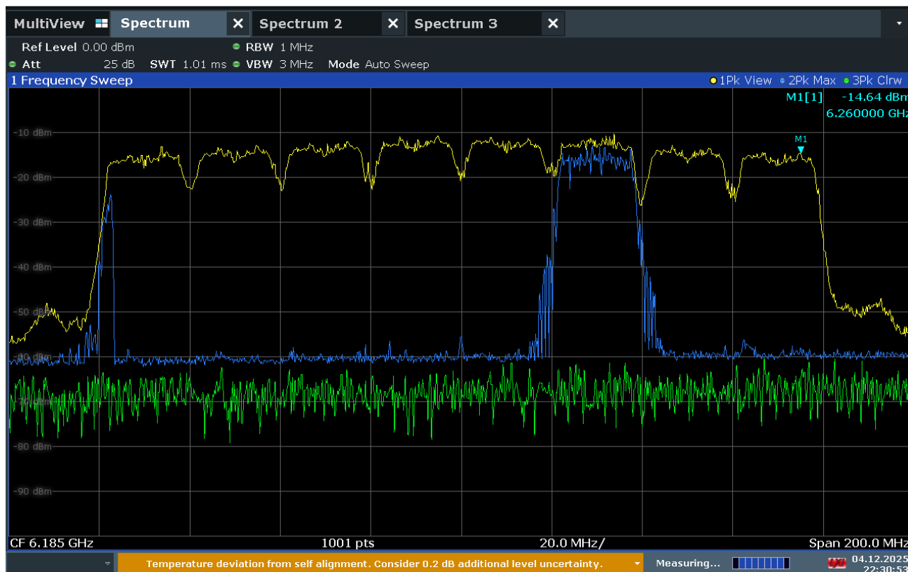
Plot 7-491. 160MHz Bandwidth, AWGN Signal Injected – 6260MHz
