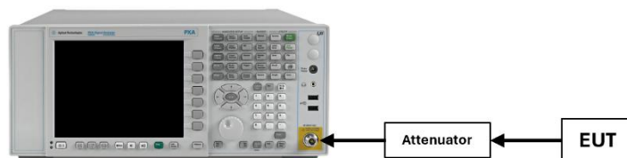
Figure 7-2. Test Instrument & Measurement Setup
