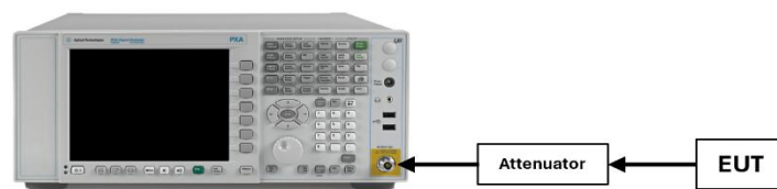
Figure 7-4. Test Instrument & Measurement Setup
