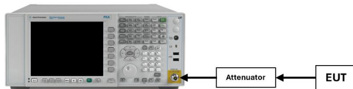
Figure 7-5. Test Instrument & Measurement Setup
