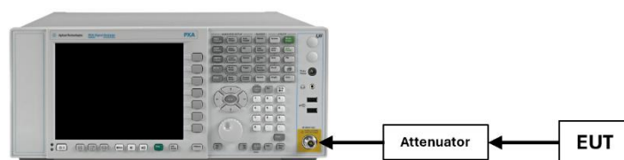
Figure 7-5. Test Instrument & Measurement Setup
