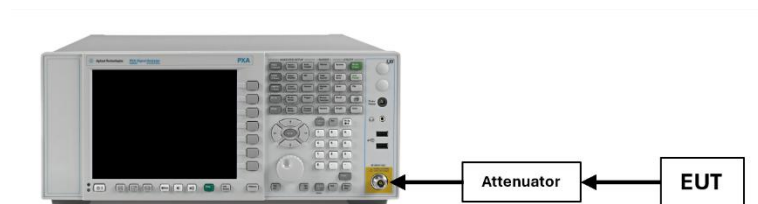
Figure 7-1. Test Instrument & Measurement Setup
