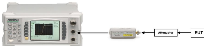
Figure 7-3. Test Instrument & Measurement Setup for Peak and Average Power Measurement
