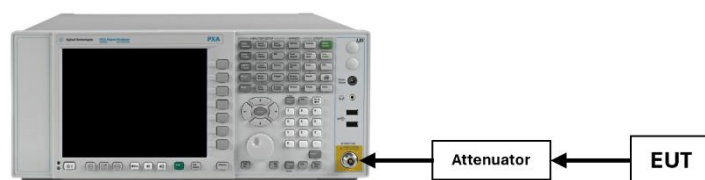
Figure 7-5. Test Instrument & Measurement Setup
